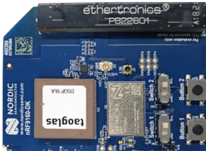
Figure 12: nRF9160 Development Kit antenna
