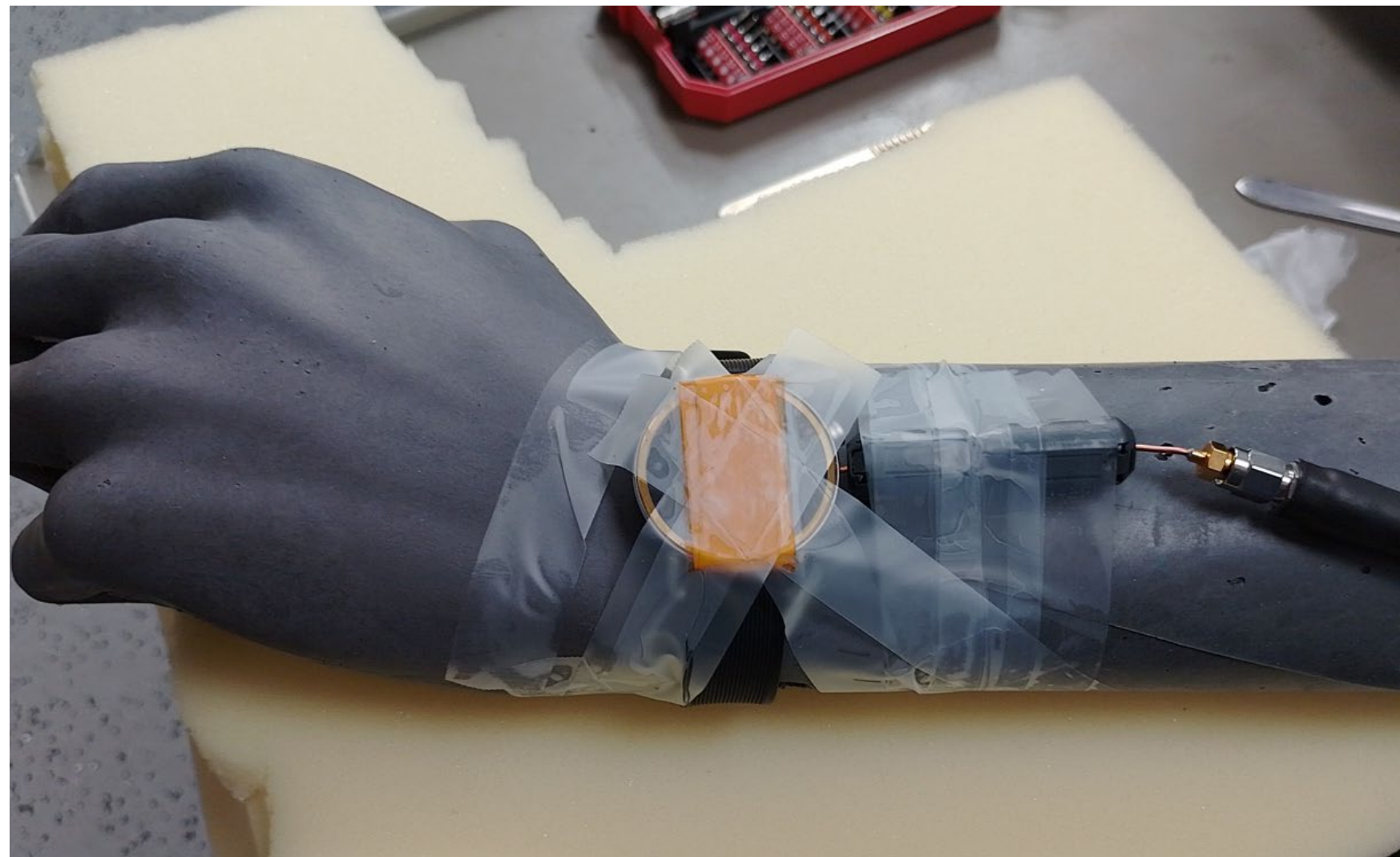
S11 measurement setup
