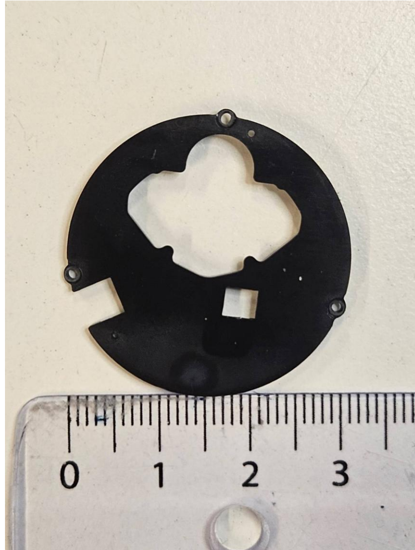
Antenna frame front
