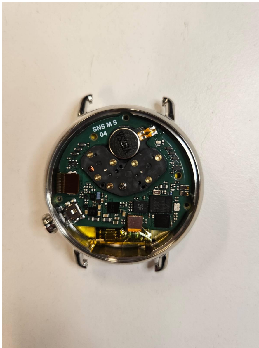
Main PCB assembled
