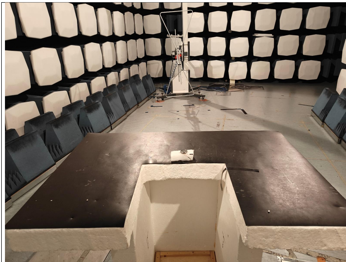
Picture 68, Radiated Spurious Emission, common setup, TX, 30 – 1000 MHz, back
