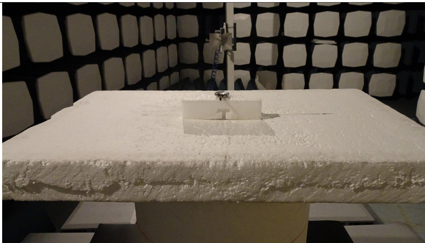
Picture 79, Radiated Spurious Emission, common setup, TX, 1 – 18 GHz, back
