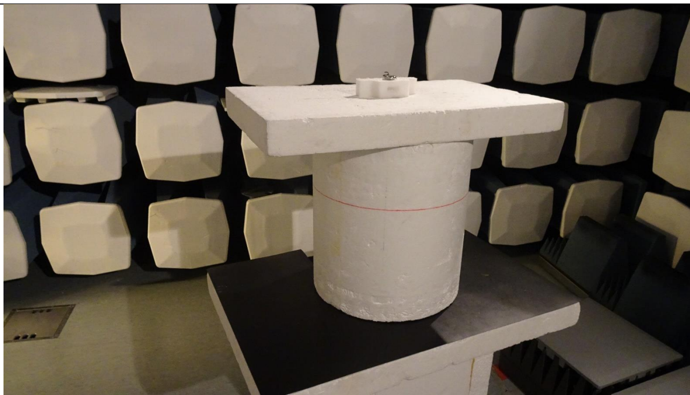
Picture 46, Radiated Spurious Emission, EUT setup, TX, 1 – 26 GHz
