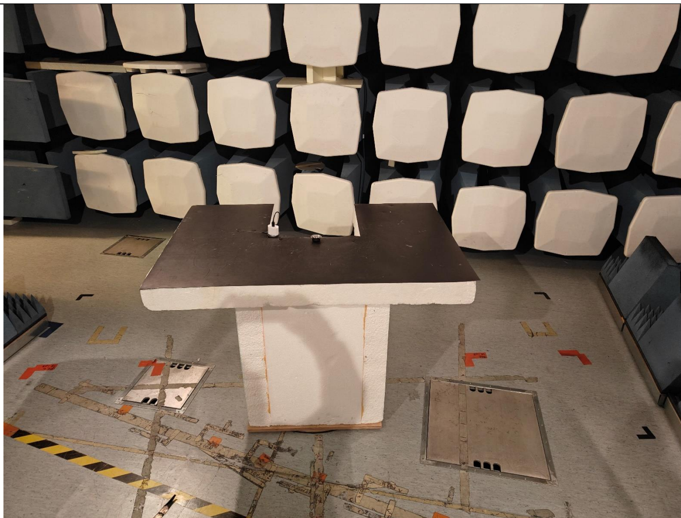
Picture 57, Radiated Spurious Emission, EUT setup, RX, 30 MHz – 12,75 GHz
