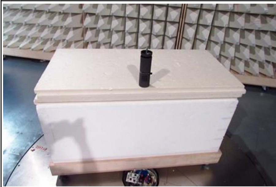
Setup for measurements below 1 GHz
