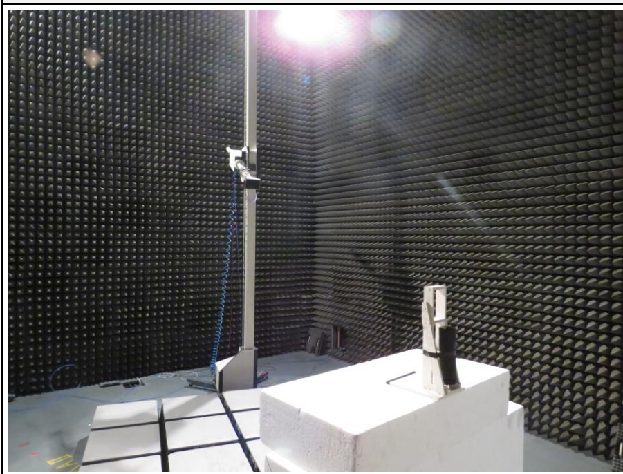
Setup for measurements above 1 GHz
