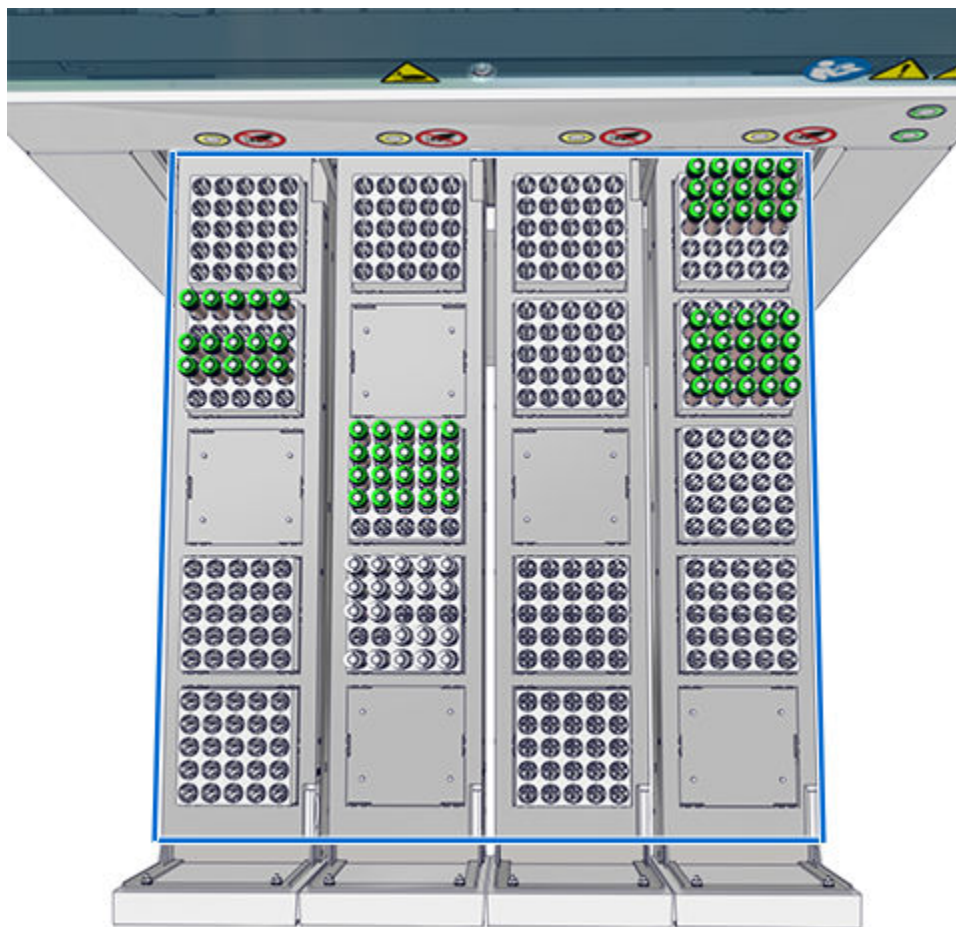
Figure 18: Sample tubes in FlexRacks in the module drawer
