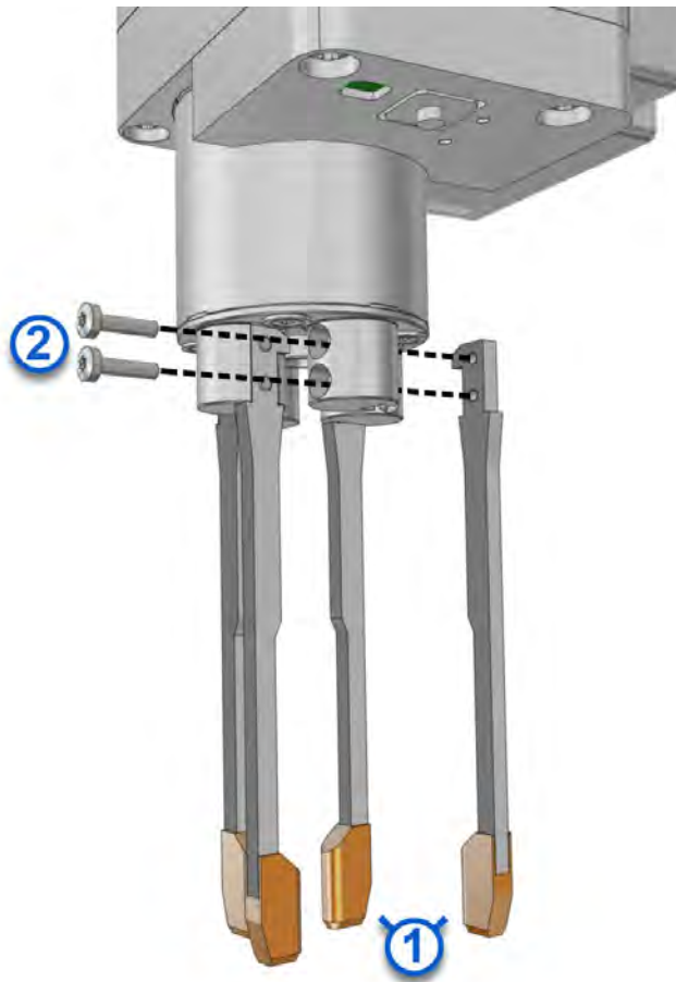
Figure 45: Robot gripper fingers and screws
