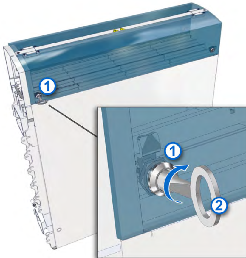
Figure 22: Track hood lock and key
