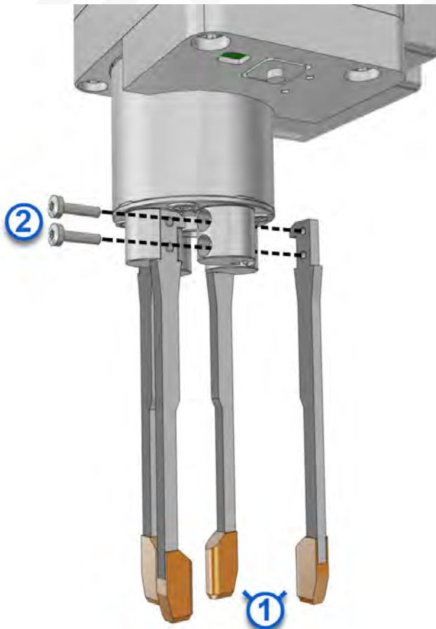
Figure 44: Replacing the robot gripper fingers
