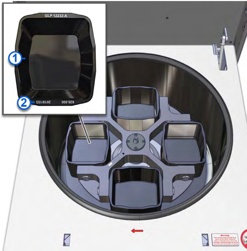
Figure 43: Correct insertion of the Bucket holders
