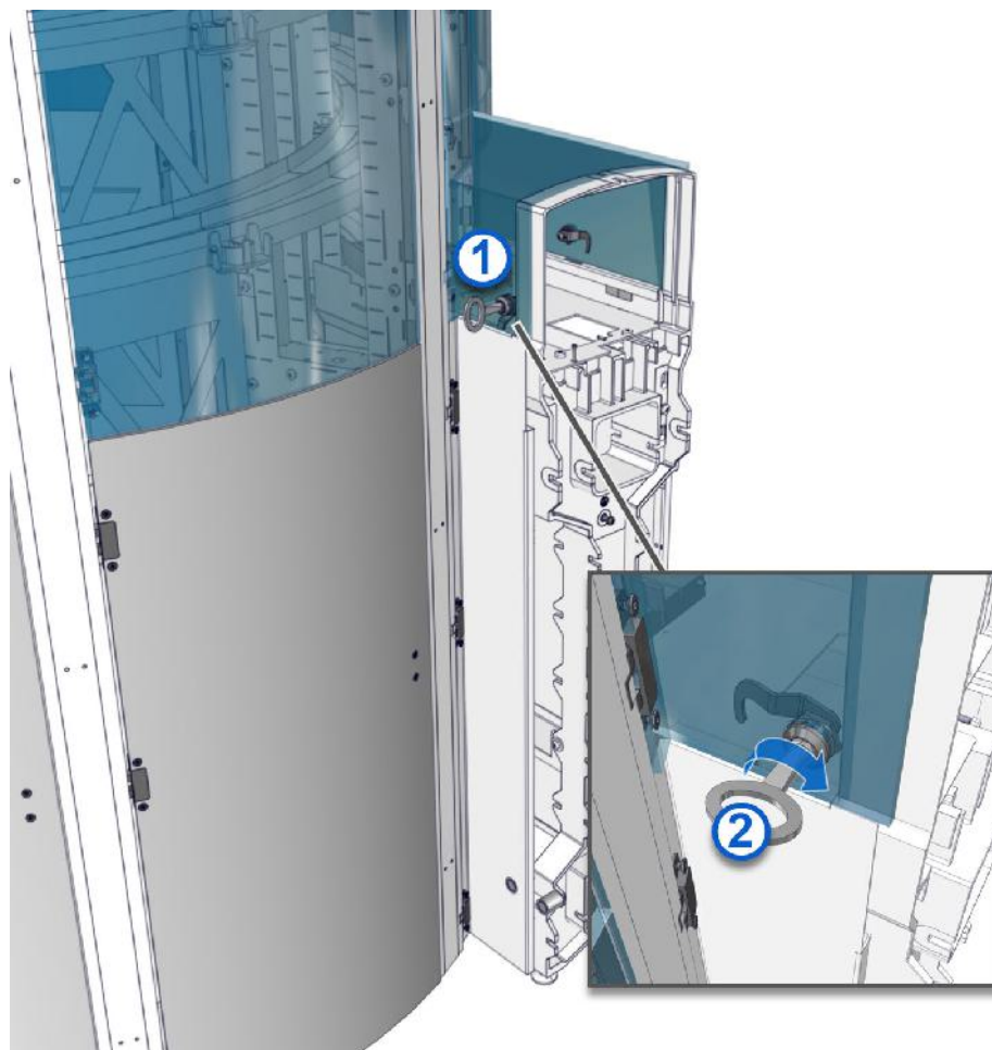
Figure 29: Track hood rear lock and key
