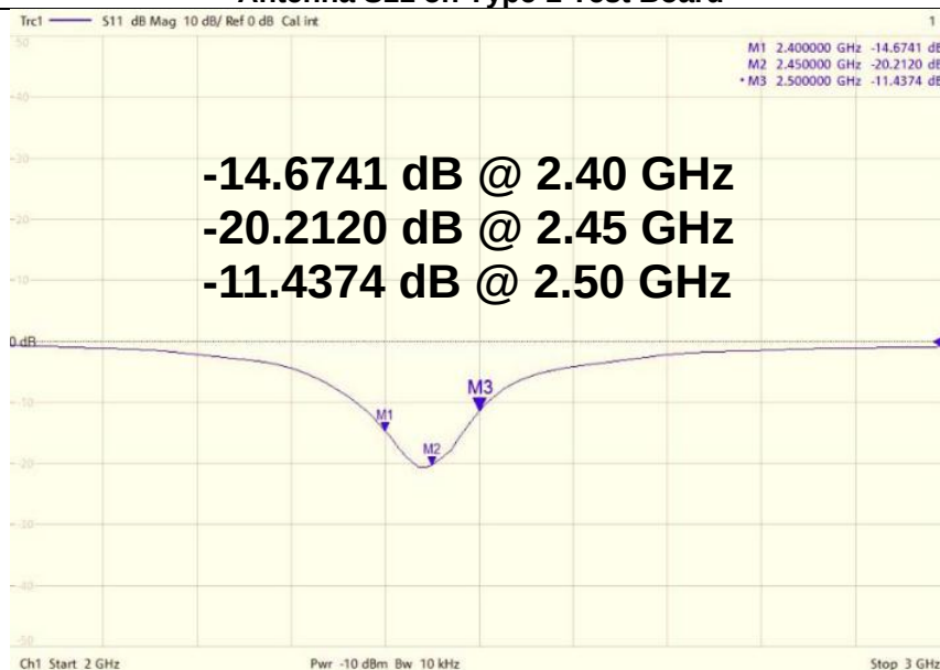
Antenna VSWR on Type-2 Test Board
