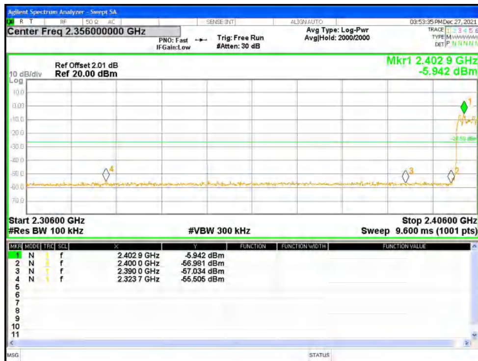
Band Edge(Hopping) NVNT 3-DH1 2480MHz Ant1 Hopping Ref
