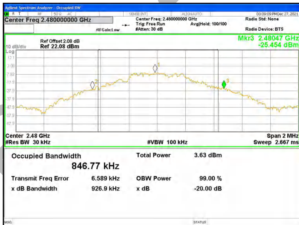
-20dB Bandwidth NVNT 2-DH1 2402MHz Ant1
