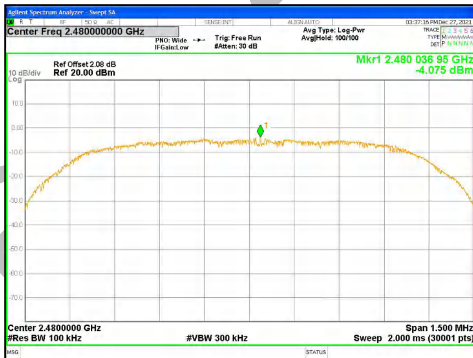
Tx. Spurious NVNT 2-DH1 2480MHz Ant1 Emission
