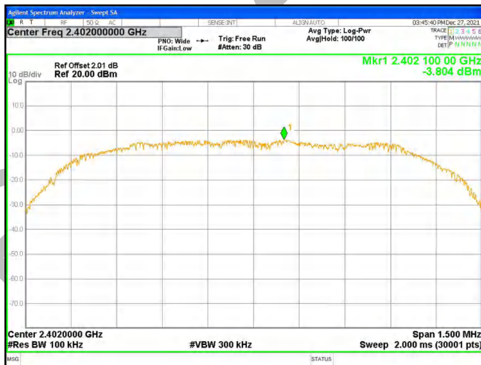
Tx. Spurious NVNT 3-DH1 2402MHz Ant1 Emission
