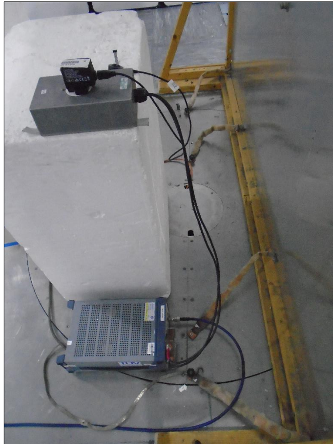
Figure 68 - AC Line Conducted Emissions
