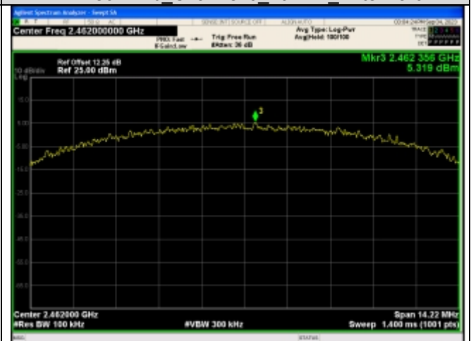
In-Band Reference Level IEEE 802.11b_Channel 11_20MHz_Antenna 0
