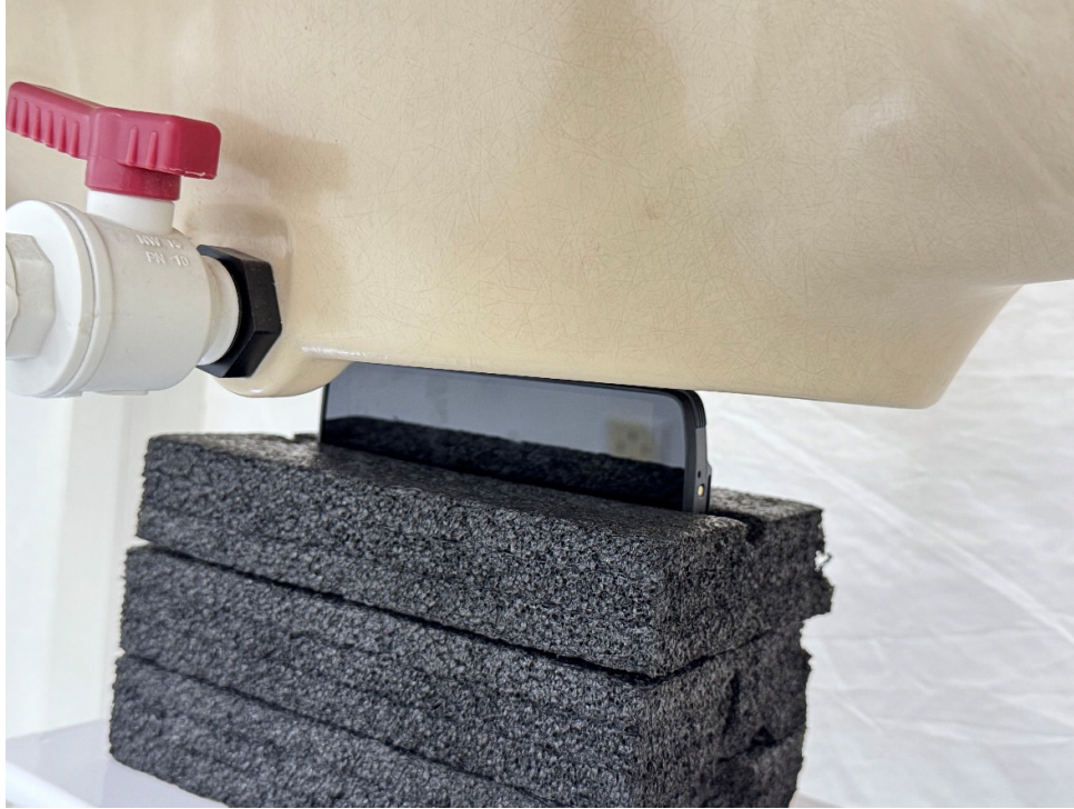
Picture 9: Right Edge, the distance from EUT to the bottom of the Phantom is 0mm
