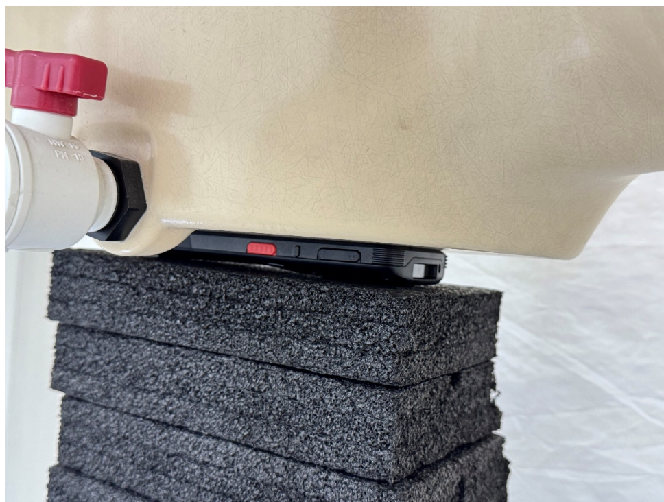
Picture 8: Front Side, the distance from EUT to the bottom of the Phantom is 0mm
