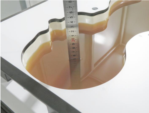
15 cm Depth Head Tissue for ELI Phantom
