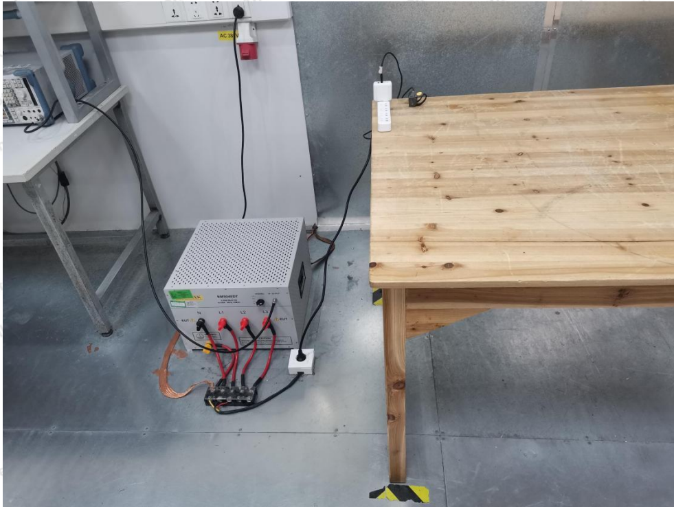
Photo of Conducted Emission Measurement
