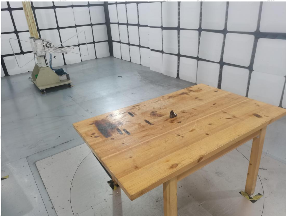
Photo of Radiation Emission Test
