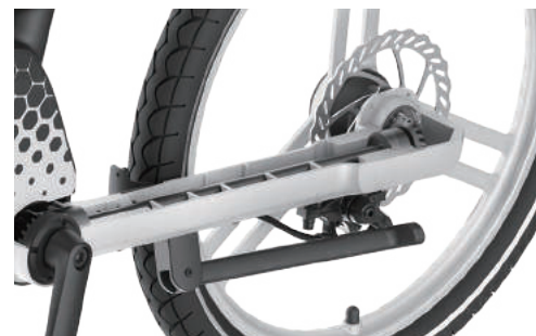
Honbike Patented Drive Shaft Fully enclosed drivetrain Easy Maintenance
