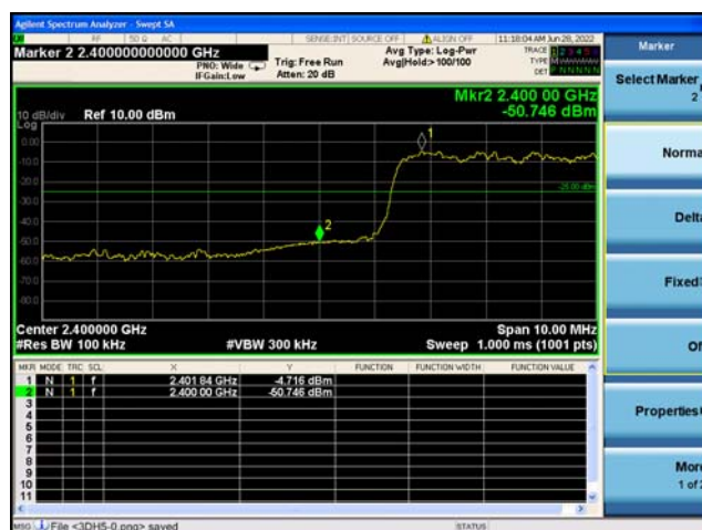
Left Band edge hopping on
