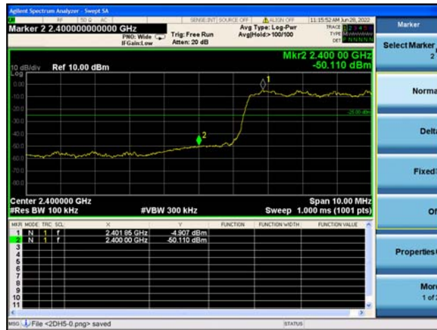
Left Band edge hopping on
