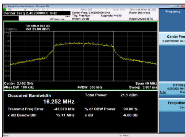
6dB Bandwidth-802.11g,2462MHz,Ant0
