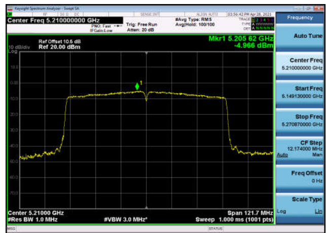
U-NII-2a Power spectral density-802.1 1n(20MHz),5300MHz,Ant1
