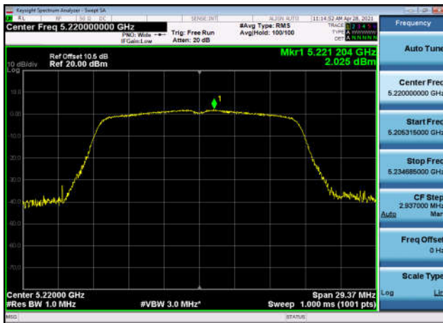
U-NII-1 Power spectral density-802.11 ac(20MHz),5180MHz,Ant1
