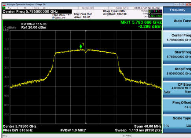
U-NII-3 Power spectral density-802.11 ac(20MHz),5745MHz,Ant1
