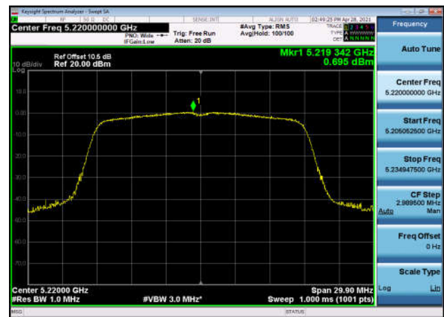
U-NII-1 Power spectral density-802.11 ac(40MHz),5190MHz,Ant1
