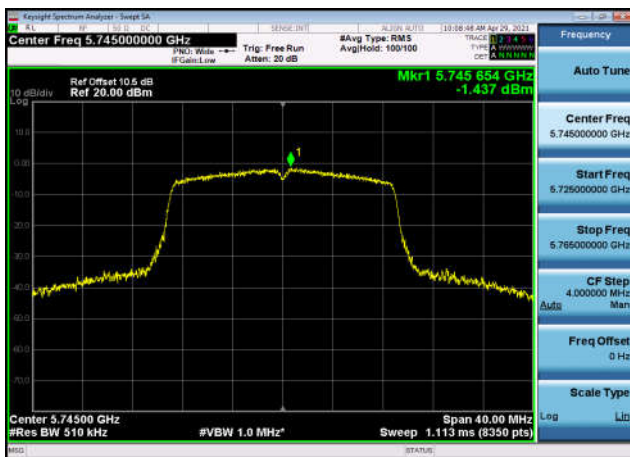
U-NII-3 Power spectral density-802.11 ac(20MHz),5825MHz,Ant1
