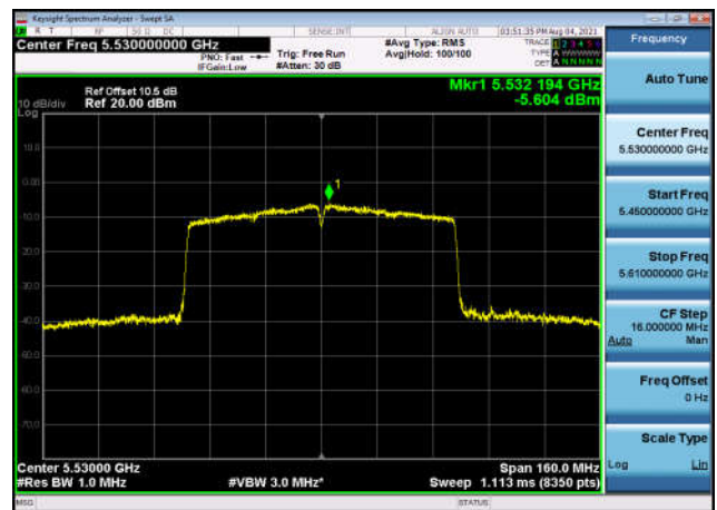
U-NII-2c Power spectral density-802.1 1ac(80MHz),5530MHz,Ant1
