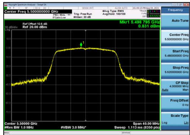
U-NII-2c Power spectral density-802.1 1a(20MHz),5700MHz,Ant1
