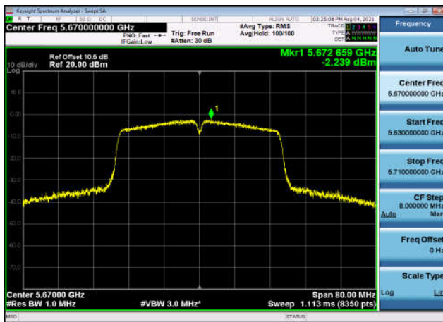
U-NII-2c Power spectral density-802.1 1a(20MHz),5580MHz,Ant1
