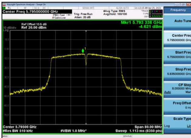
U-NII-3 Power spectral density-802.11 ac(40MHz),5795MHz,Ant1
