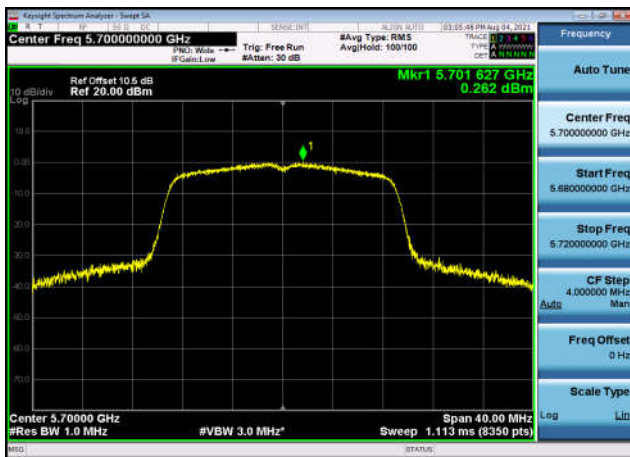
U-NII-2c Power spectral density-802.1 1ac(40MHz),5670MHz,Ant1
