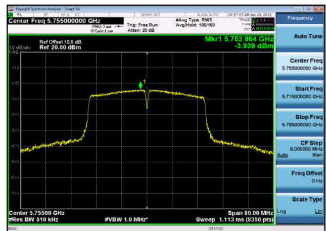
U-NII-3 Power spectral density-802.11 ac(40MHz),5755MHz,Ant1
