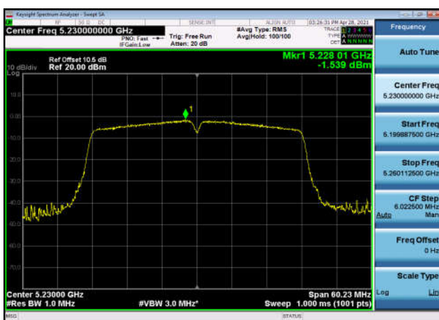
U-NII-1 Power spectral density-802.11 n(40MHz),5230MHz,Ant1
