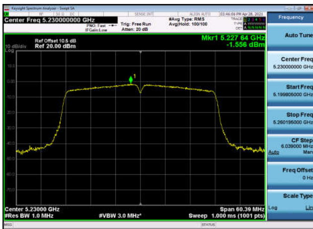
U-NII-2a Power spectral density-802.1 1n(20MHz),5260MHz,Ant1
