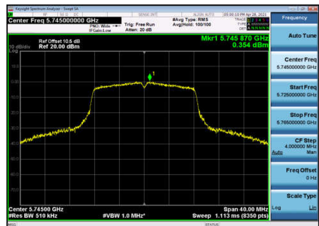
U-NII-3 Power spectral density-802.11 a(20MHz),5745MHz,Ant1
