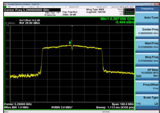
U-NII-2c Power spectral density-802.1 1n(20MHz),5580MHz,Ant1
