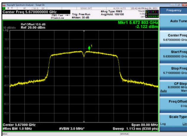
U-NII-2c Power spectral density-802.1 1ac(40MHz),5670MHz,Ant1
