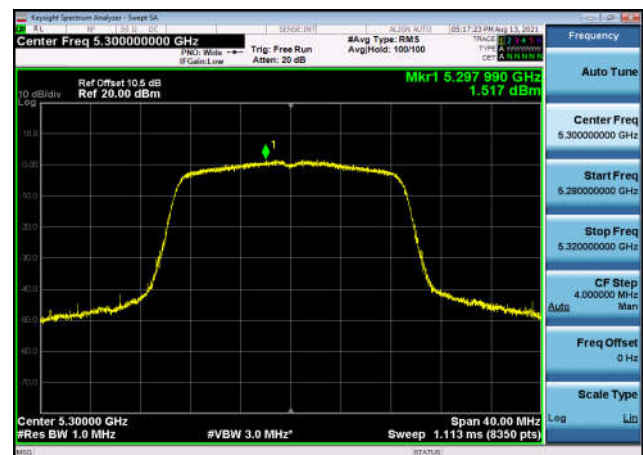
U-NII-2a Power spectral density-802.1 1ac(20MHz),5300MHz,Ant1
