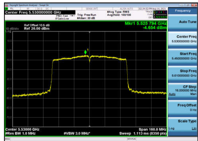
U-NII-2c Power spectral density-802.1 1ac(80MHz),5530MHz,Ant1
