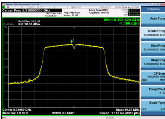
U-NII-2c Power spectral density-802.1 1n(20MHz),5500MHz,Ant1
