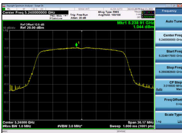
U-NII-1 Power spectral density-802.11 n(40MHz),5230MHz,Ant1
