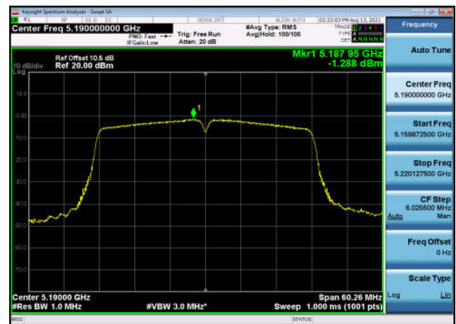
U-NII-1 Power spectral density-802.11 ac(40MHz),5190MHz,Ant1
