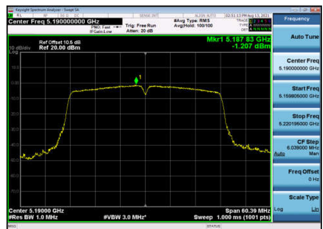
U-NII-1 Power spectral density-802.11 a(20MHz),5180MHz,Ant1
