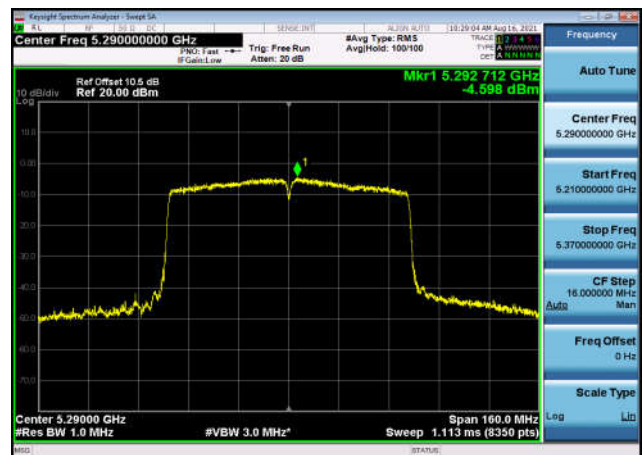
U-NII-2c Power spectral density-802.1 1n(20MHz),5580MHz,Ant1
