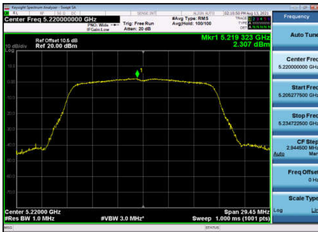
U-NII-1 Power spectral density-802.11 ac(20MHz),5180MHz,Ant1
