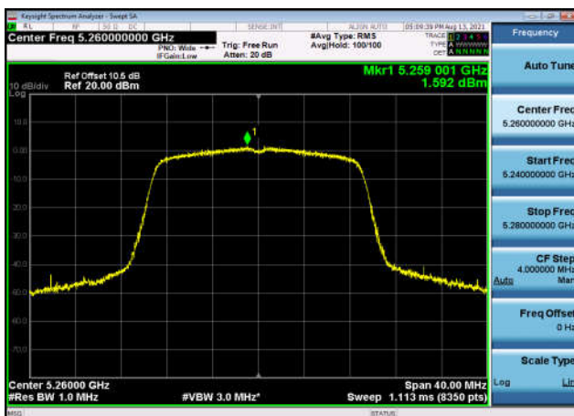
U-NII-2a Power spectral density-802.1 1ac(20MHz),5260MHz,Ant1
