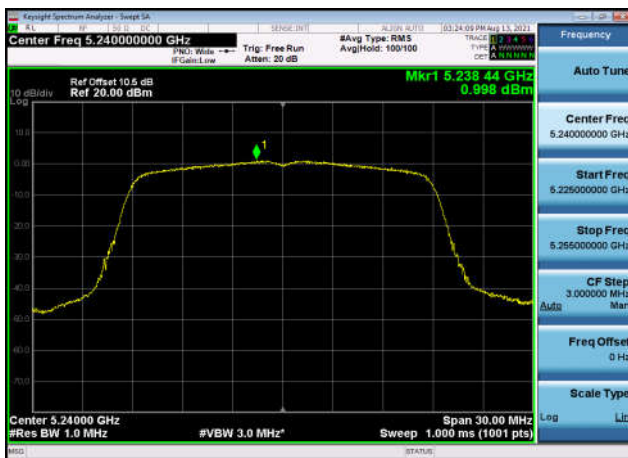
U-NII-1 Power spectral density-802.11 ac(20MHz),5240MHz,Ant1
