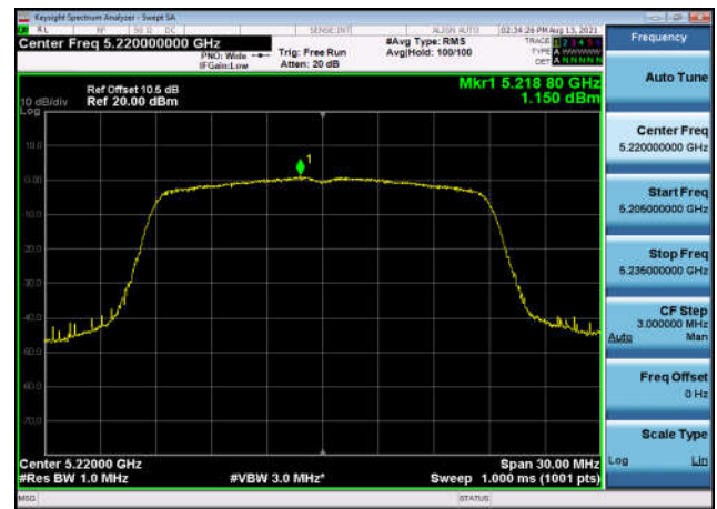
U-NII-1 Power spectral density-802.11 n(40MHz),5190MHz,Ant1
