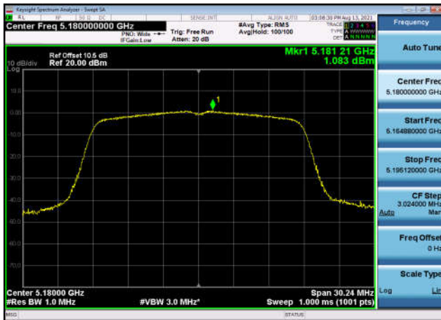
U-NII-1 Power spectral density-802.11 ac(20MHz),5240MHz,Ant1
