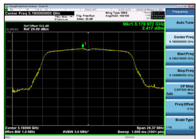
U-NII-1 Power spectral density-802.11 a(20MHz),5180MHz,Ant1
