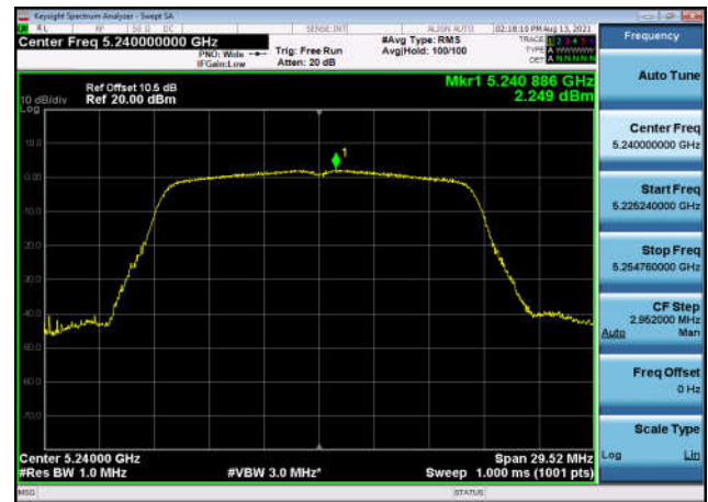
U-NII-1 Power spectral density-802.11 ac(20MHz),5220MHz,Ant1
