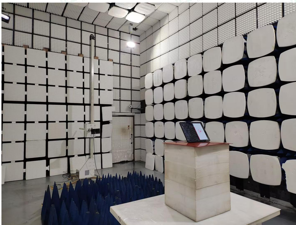
Radiated Emissions Measurement (Above 1GHz)
