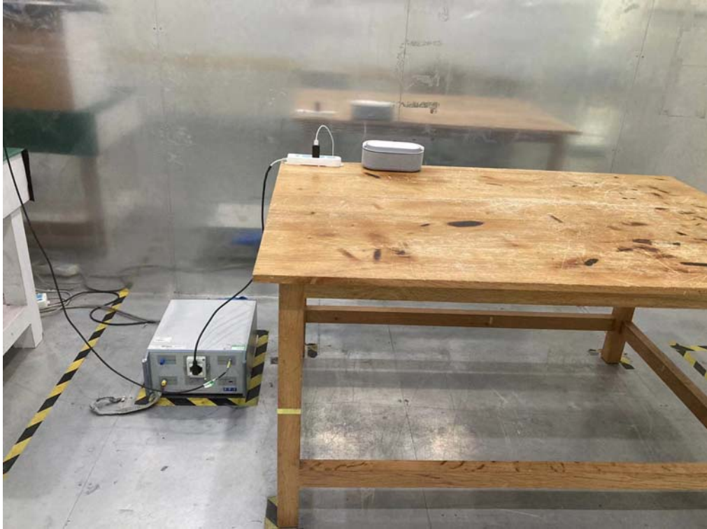
Conducted setup (Bluetooth)
