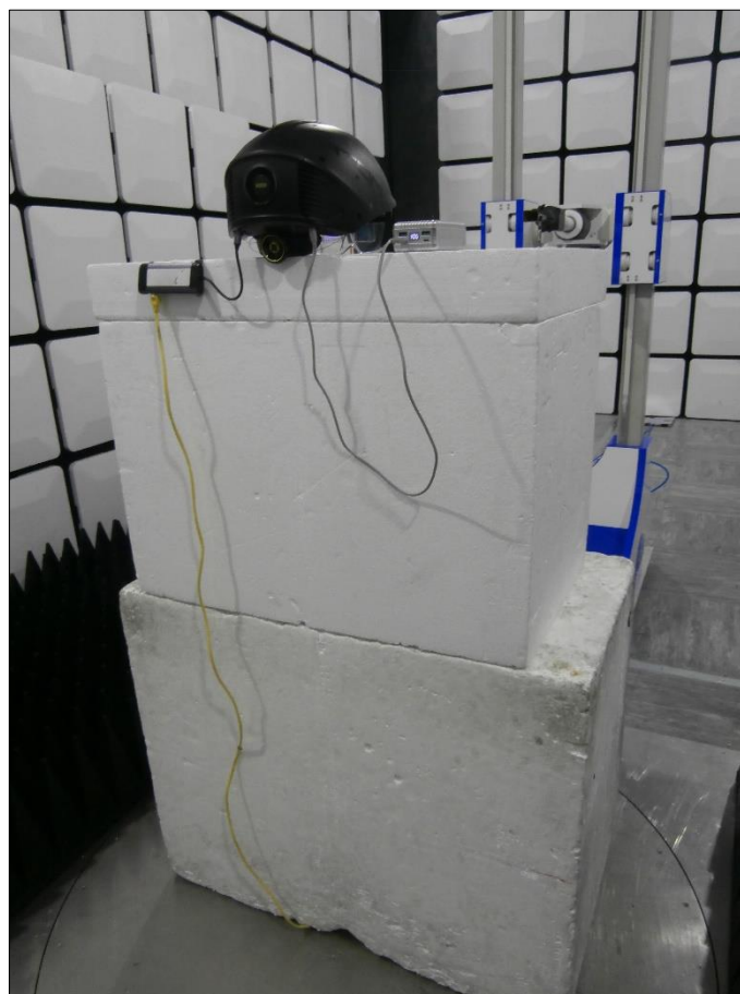
Figure 26 - Test Setup - 18 GHz to 25 GHz - X Orientation
