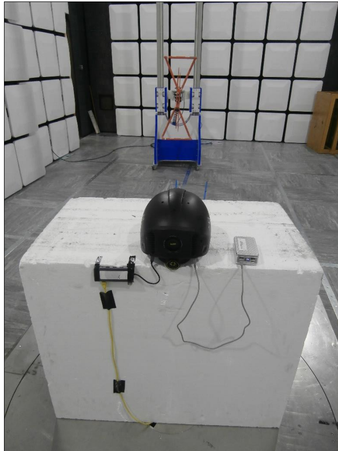
Figure 20 - Test Setup - 30 MHz to 1 GHz - X Orientation
