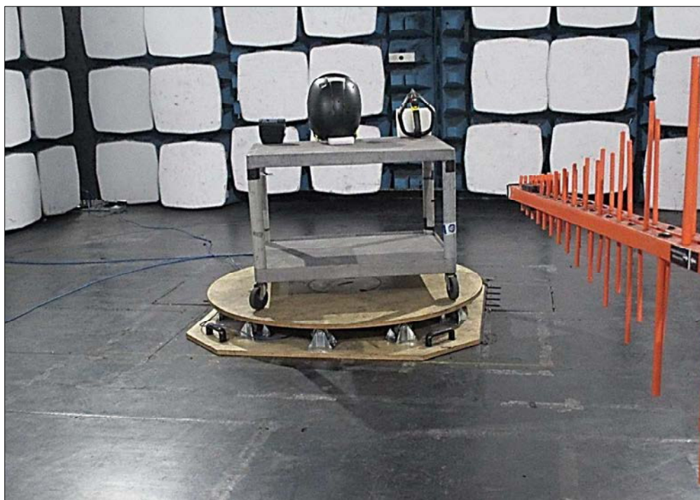
Figure 34 - Test Setup - 30 MHz to 1 GHz- Z Orientation
