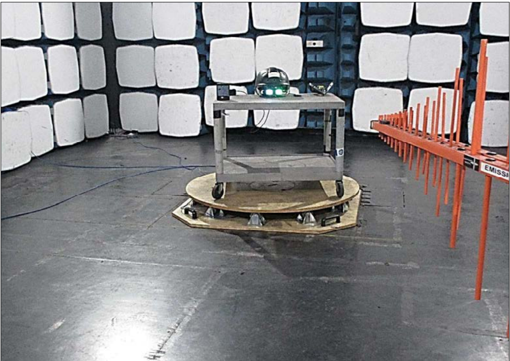
Figure 54 - Test Setup - 30 MHz to 1 GHz - X Orientation
