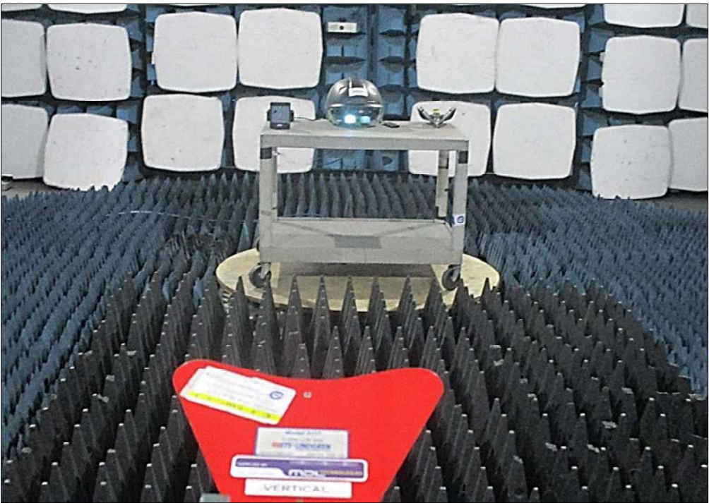
Figure 55 - Test Setup - 1 GHz to 13 GHz - X Orientation
