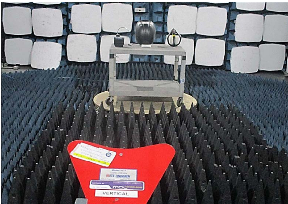
Figure 59 - Test Setup - 1 GHz to 18 GHz - Z Orientation
