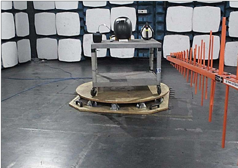
Figure 58 - Test Setup - 30 MHz to 1 GHz - Z Orientation
