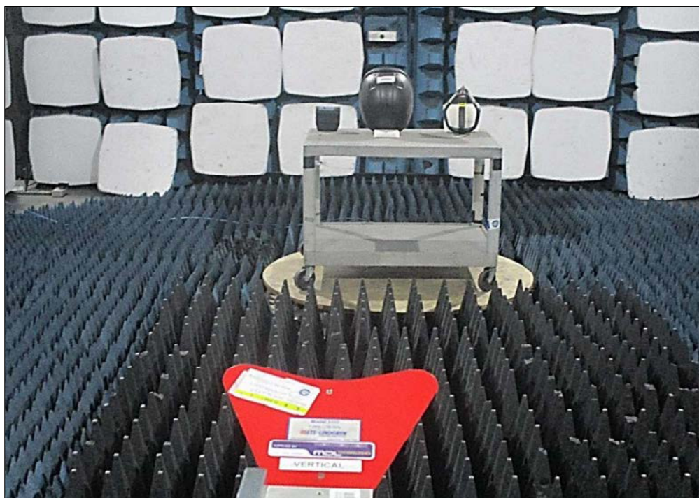
Figure 35 - Test Setup - 1 GHz to 13 GHz- Z Orientation
