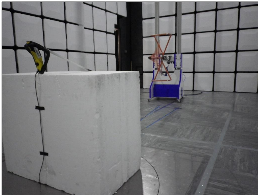
Figure 67 - Test Setup - 30 MHz to 1 GHz - Y Orientation
