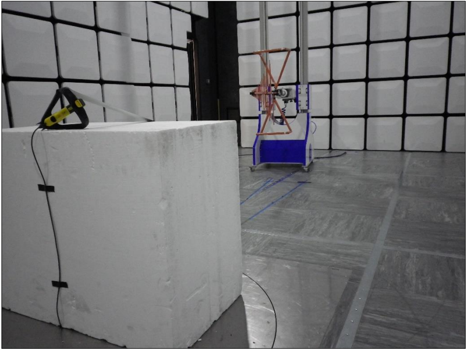
Figure 68 - Test Setup - 30 MHz to 1 GHz - Z Orientation
