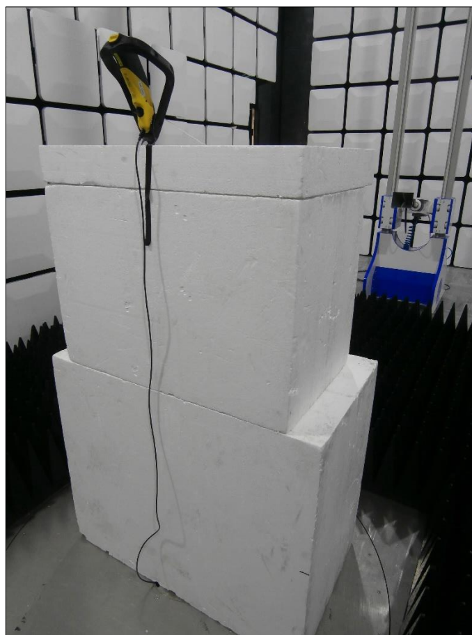
Figure 70 - Test Setup - 1 GHz to 18 GHz - Y Orientation
