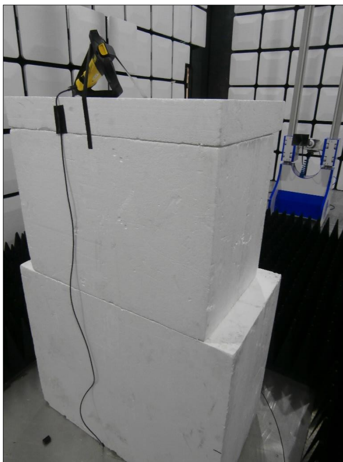
Figure 71 - Test Setup - 1 GHz to 18 GHz - Z Orientation
