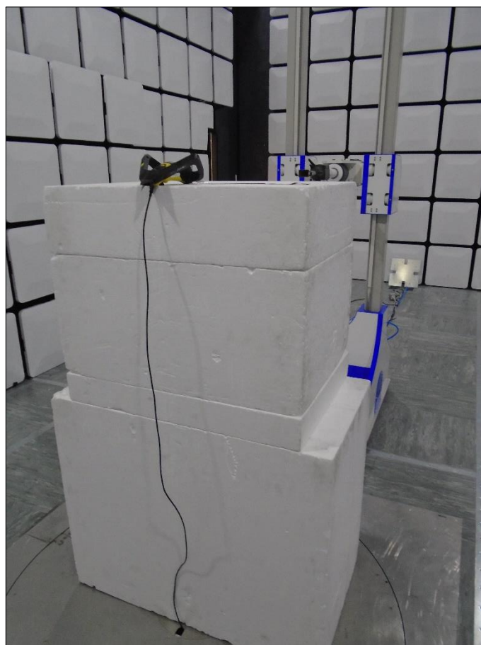
Figure 72 - Test Setup - 18 GHz to 25 GHz - X Orientation
