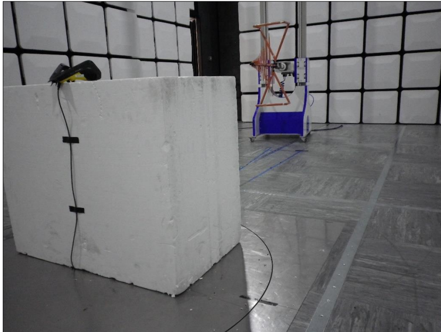
Figure 66 - Test Setup - 30 MHz to 1 GHz - X Orientation
