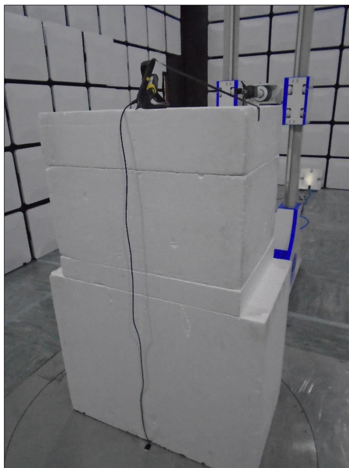
Figure 74 - Test Setup - 18 GHz to 25 GHz - Z Orientation
