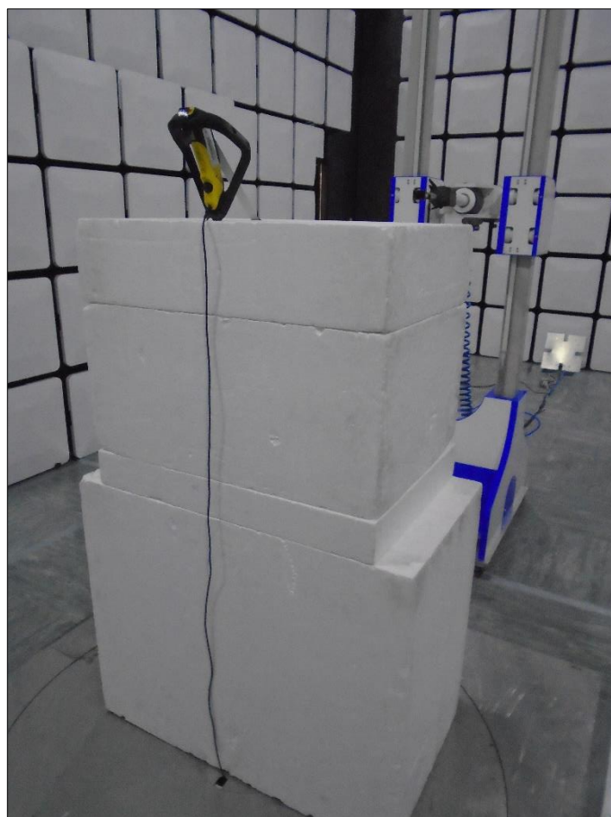
Figure 73 - Test Setup - 18 GHz to 25 GHz - Y Orientation
