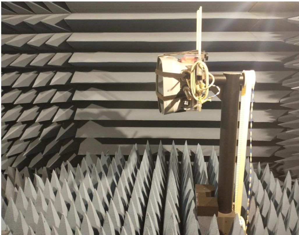
Figure 1: Measurement setup Wifi Antenna
