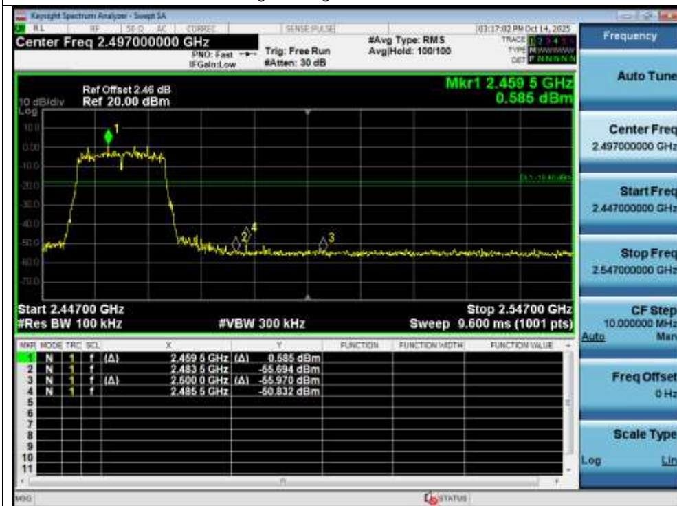
Band Edge NVNT g 2462MHz Ant1 Emission
