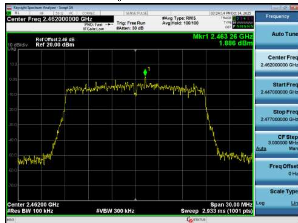
Band Edge NVNT n20 2462MHz Ant1 Emission
