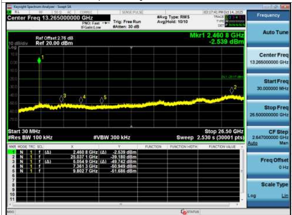
Tx. Spurious NVNT g 2462MHz Ant1 Emission
