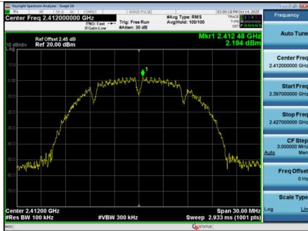
Tx. Spurious NVNT b 2412MHz Ant1 Emission
