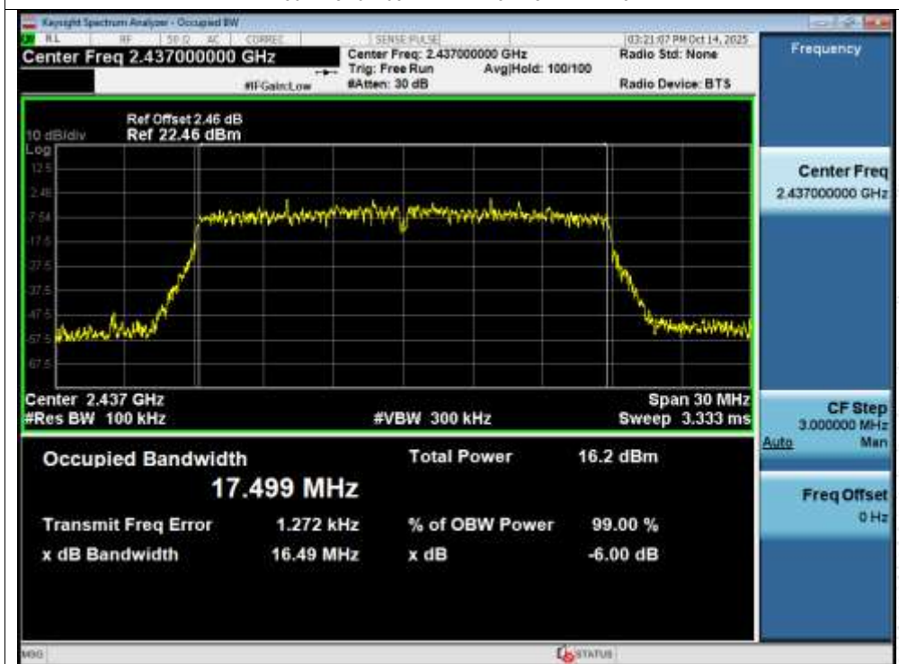
-6dB Bandwidth NVNT n20 2437MHz Ant1
