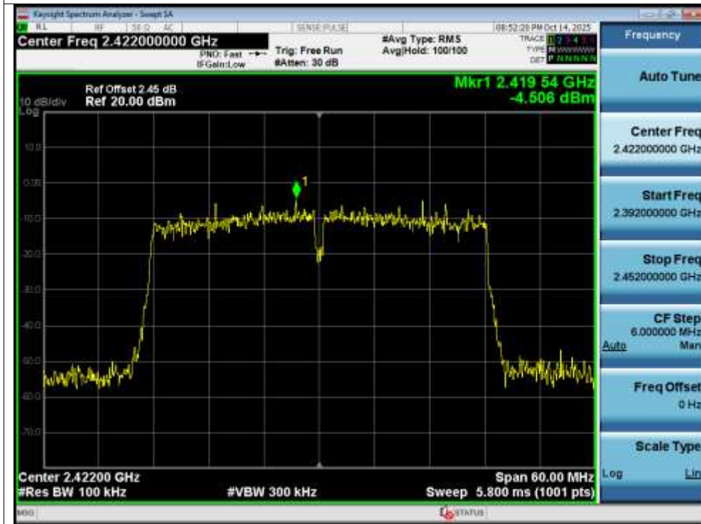
Band Edge NVNT n40 2422MHz Ant1 Emission
