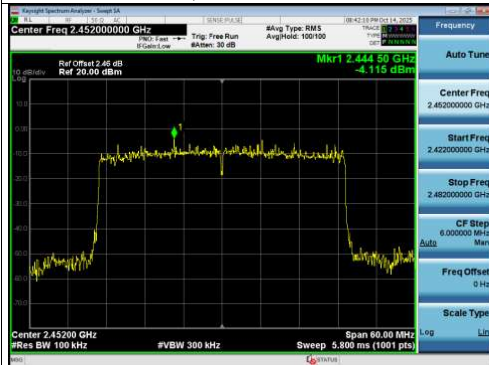
Band Edge NVNT ax40 2452MHz Ant1 Emission
