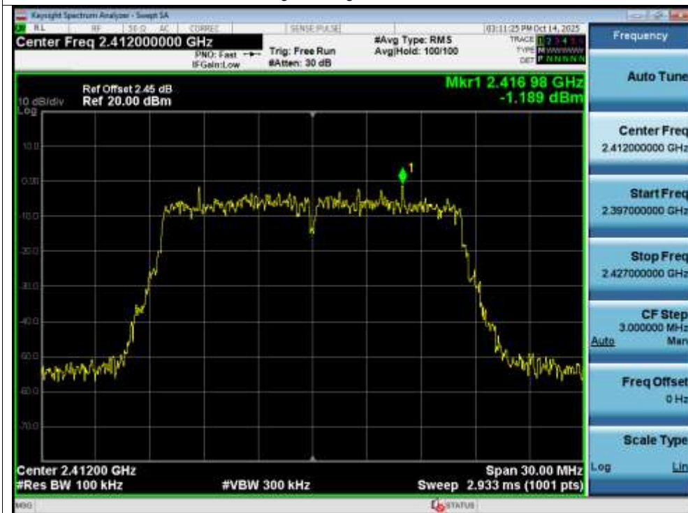
Band Edge NVNT g 2412MHz Ant1 Emission
