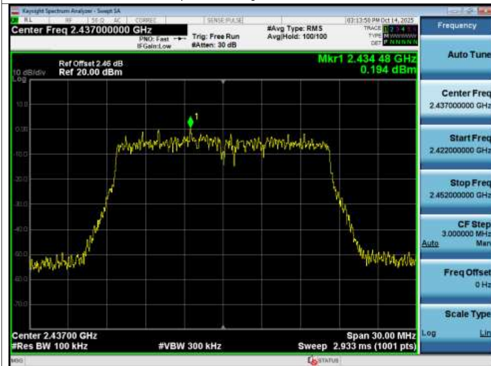
Tx. Spurious NVNT g 2437MHz Ant1 Emission
