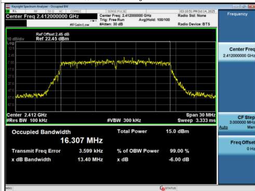
-6dB Bandwidth NVNT g 2412MHz Ant1
