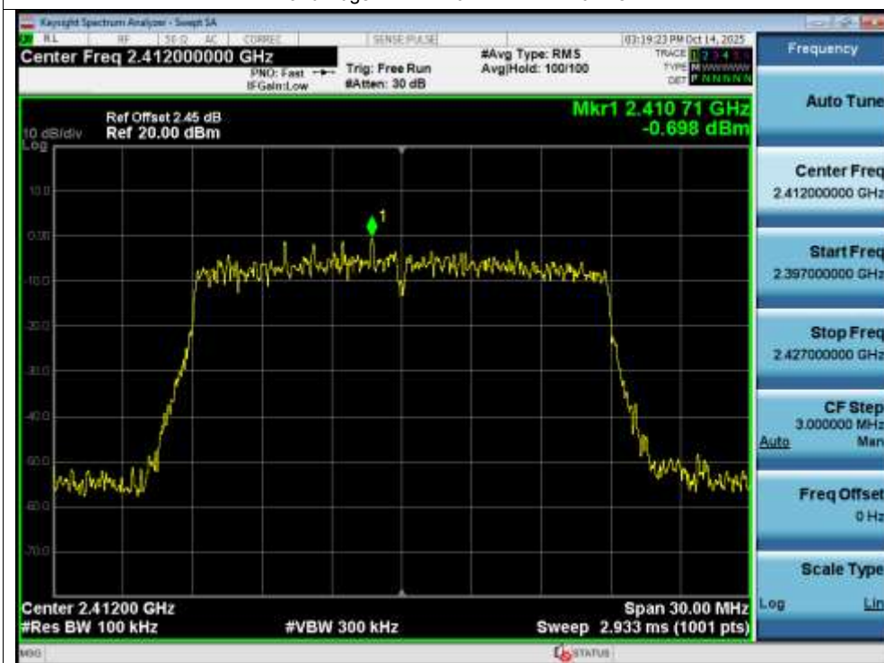
Band Edge NVNT n20 2412MHz Ant1 Emission
