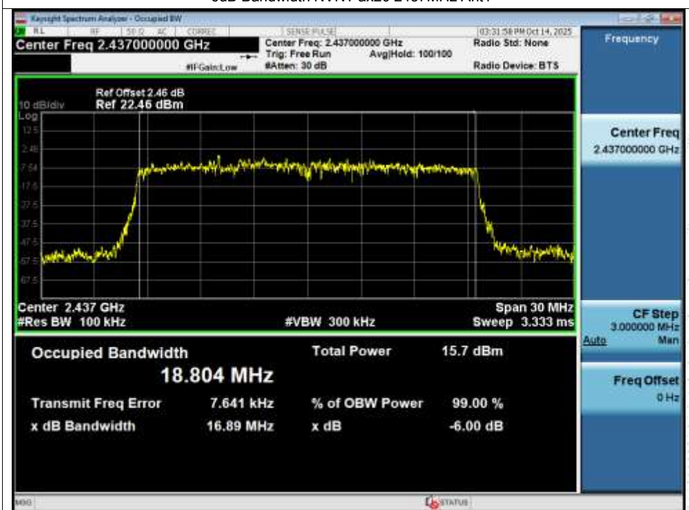
-6dB Bandwidth NVNT ax20 2437MHz Ant1
