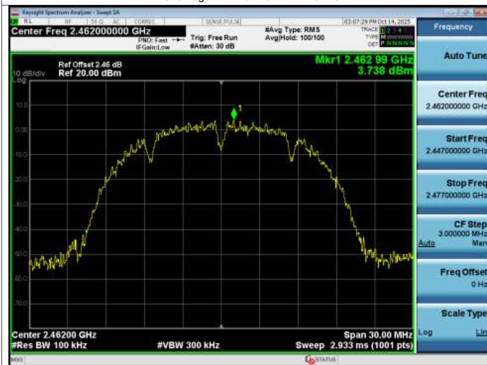
Band Edge NVNT b 2462MHz Ant1 Emission
