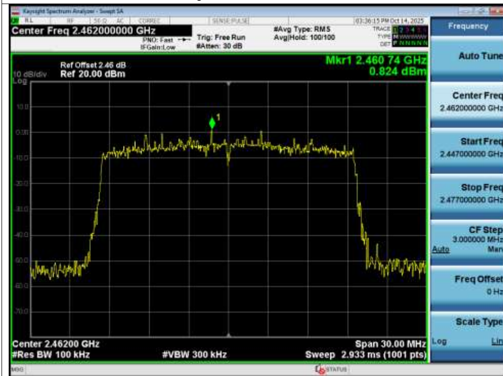
Band Edge NVNT ax20 2462MHz Ant1 Emission
