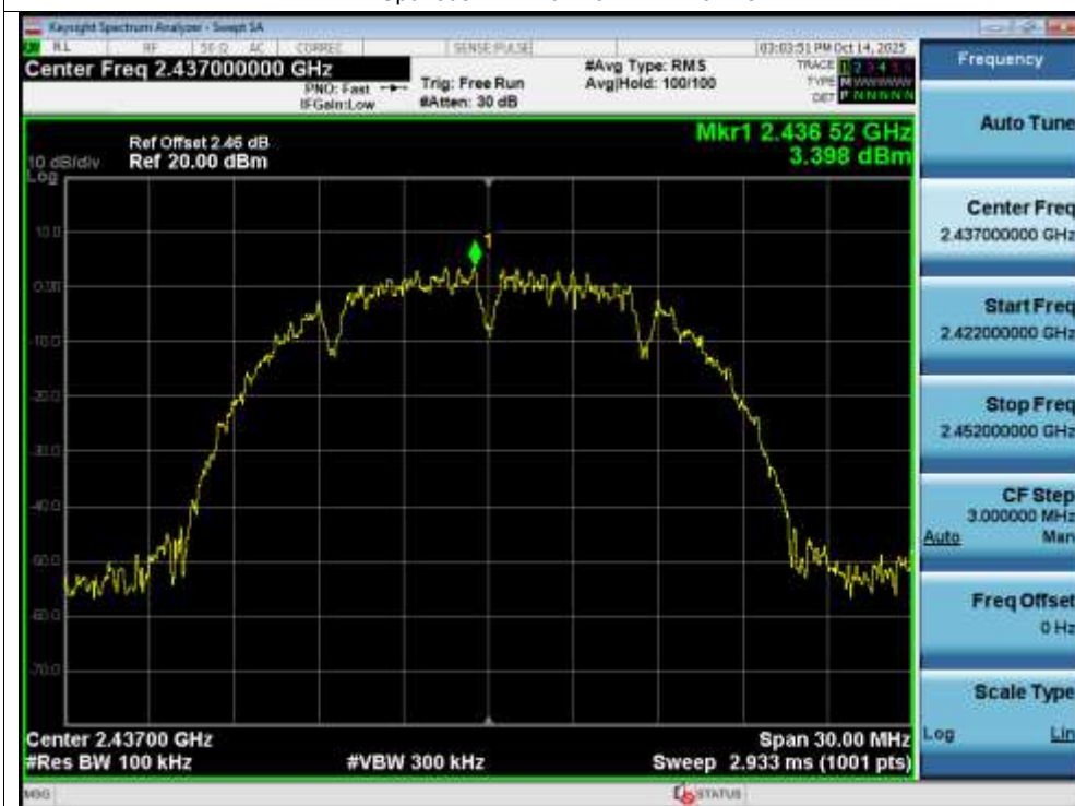
Tx. Spurious NVNT b 2437MHz Ant1 Emission
