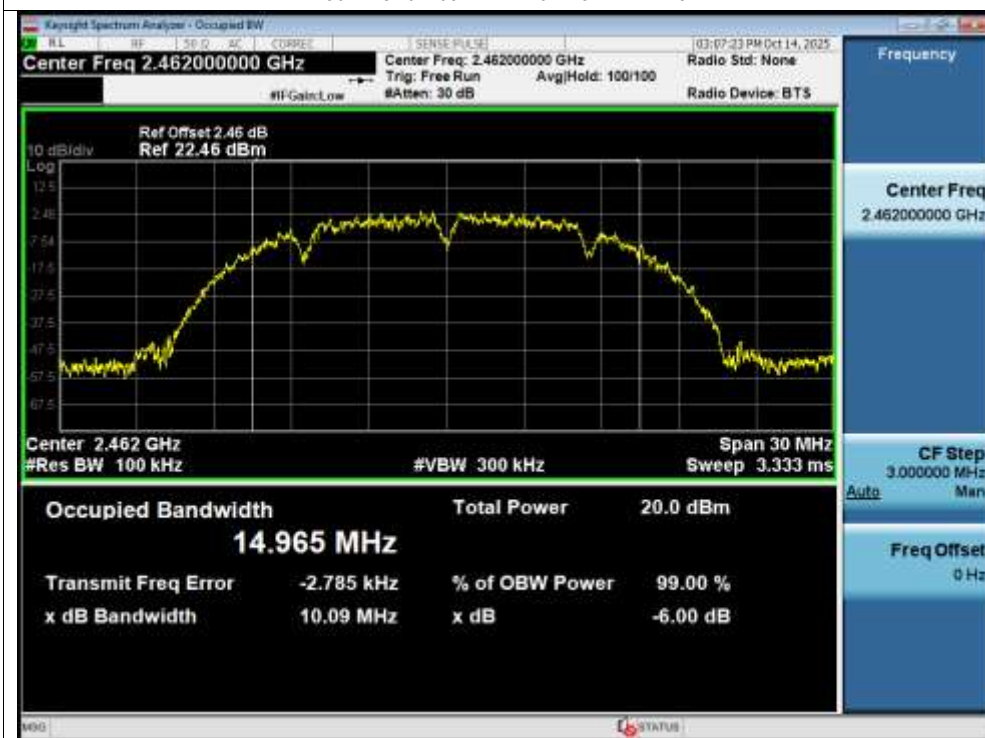
-6dB Bandwidth NVNT g 2412MHz Ant1
