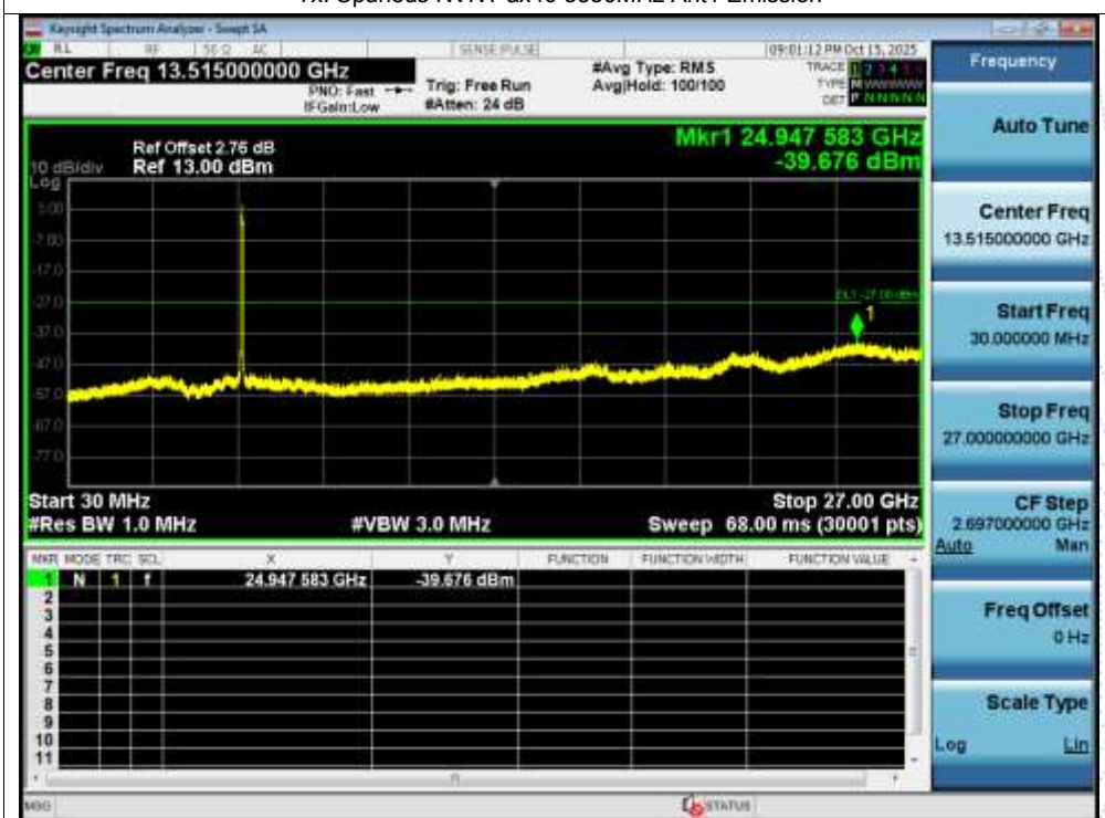
Tx. Spurious NVNT ax40 5550MHz Ant1 Emission
