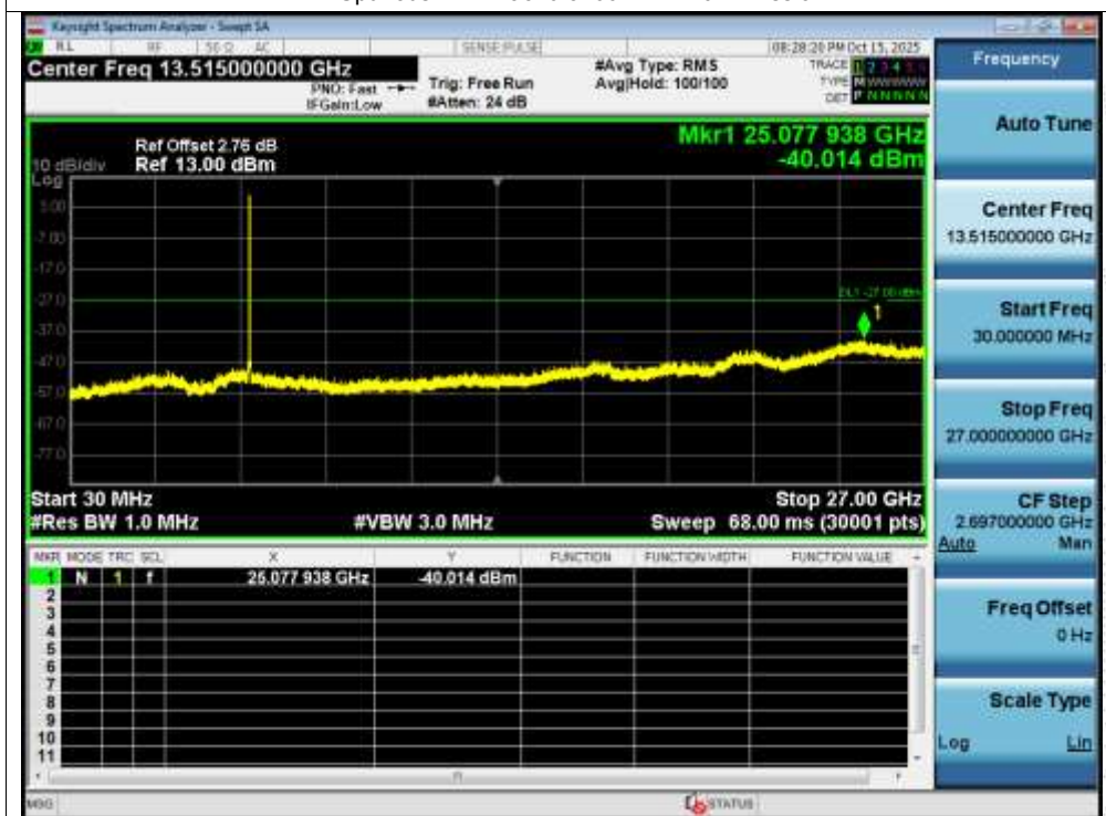
Tx. Spurious NVNT ac20 5700MHz Ant1 Emission
