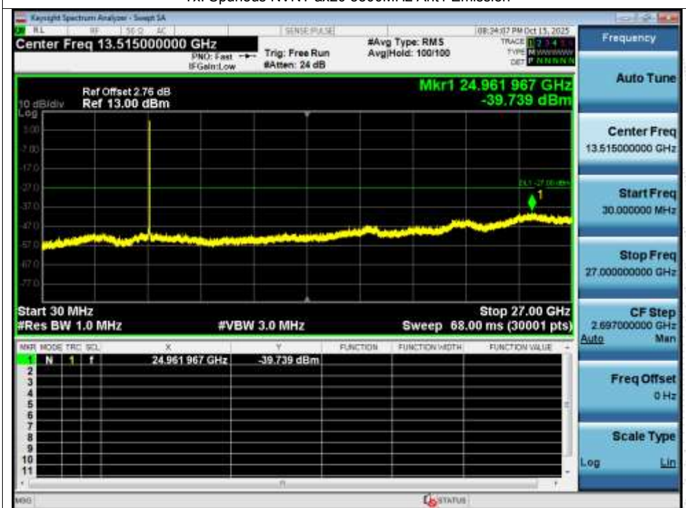
Tx. Spurious NVNT ax20 5500MHz Ant1 Emission
