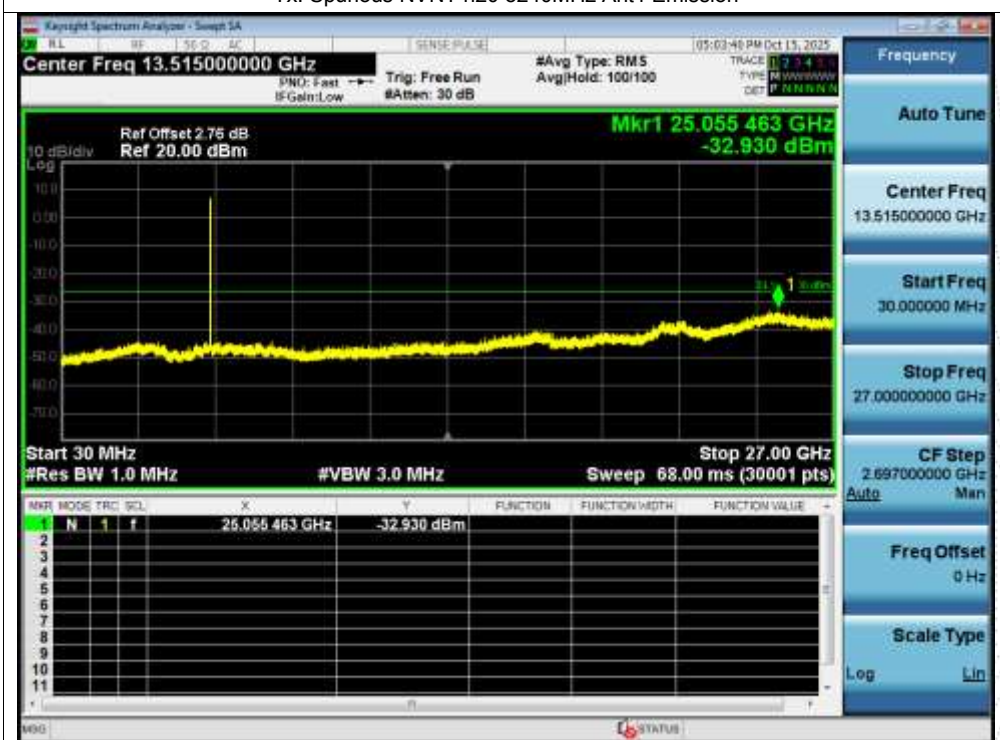
Tx. Spurious NVNT n20 5240MHz Ant1 Emission
