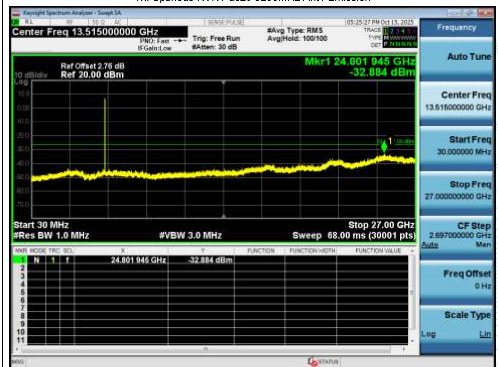
Tx. Spurious NVNT ac20 5200MHz Ant1 Emission
