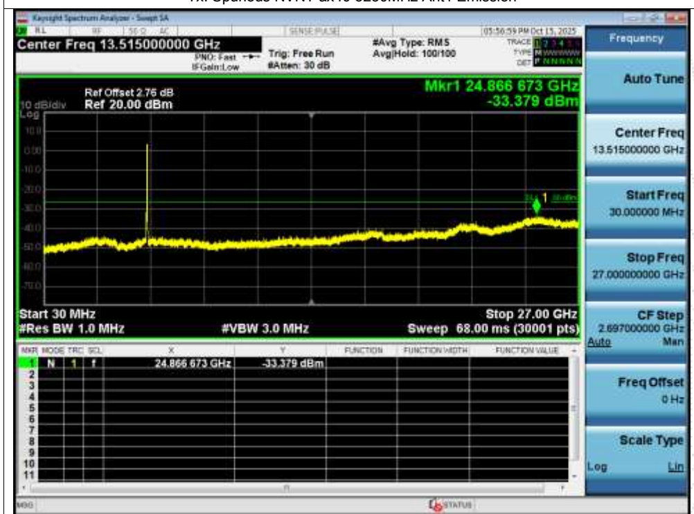
Tx. Spurious NVNT ax40 5230MHz Ant1 Emission
