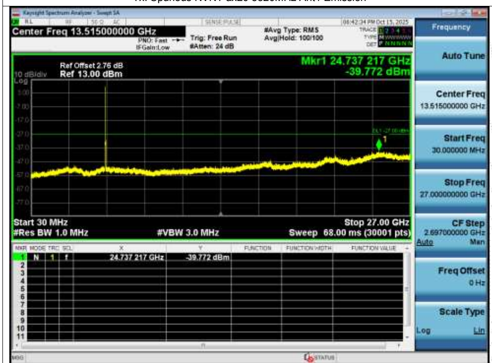
Tx. Spurious NVNT ax20 5320MHz Ant1 Emission
