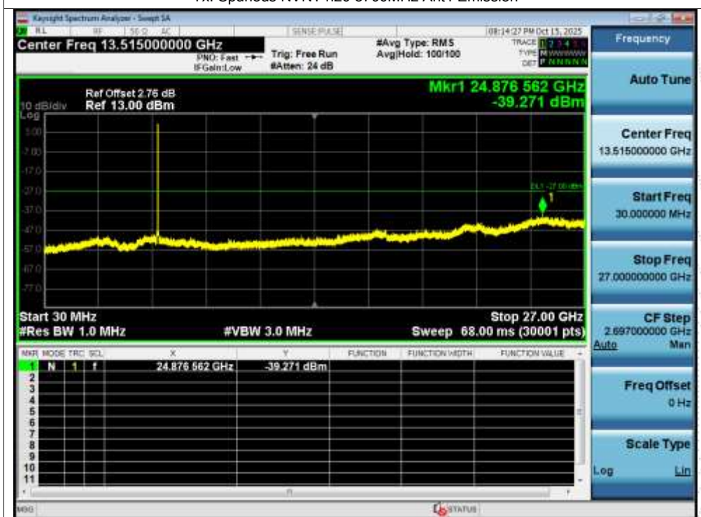
Tx. Spurious NVNT n20 5700MHz Ant1 Emission
