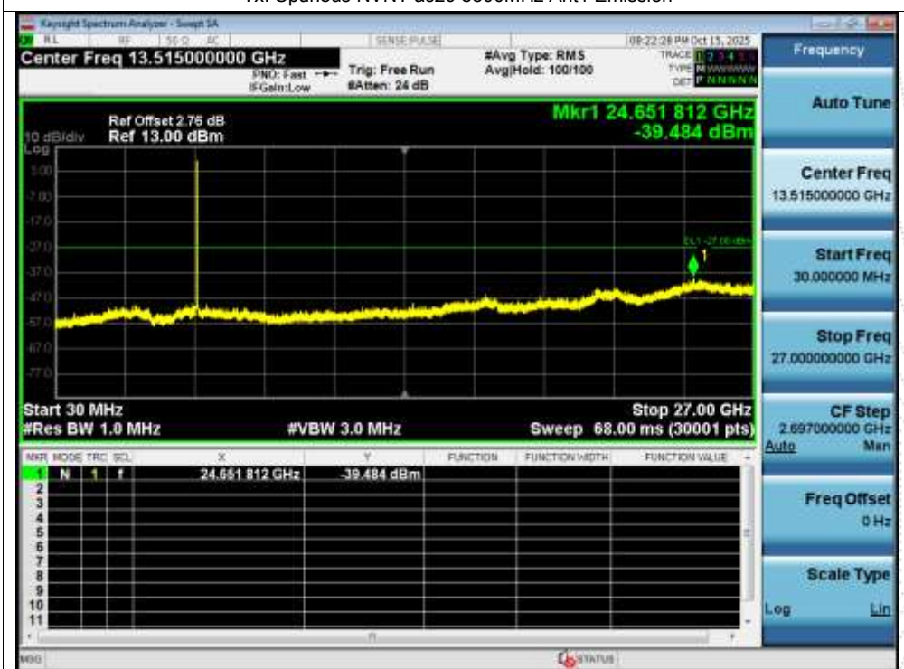
Tx. Spurious NVNT ac20 5500MHz Ant1 Emission
