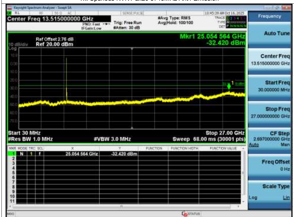
Tx. Spurious NVNT ax20 5745MHz Ant1 Emission
