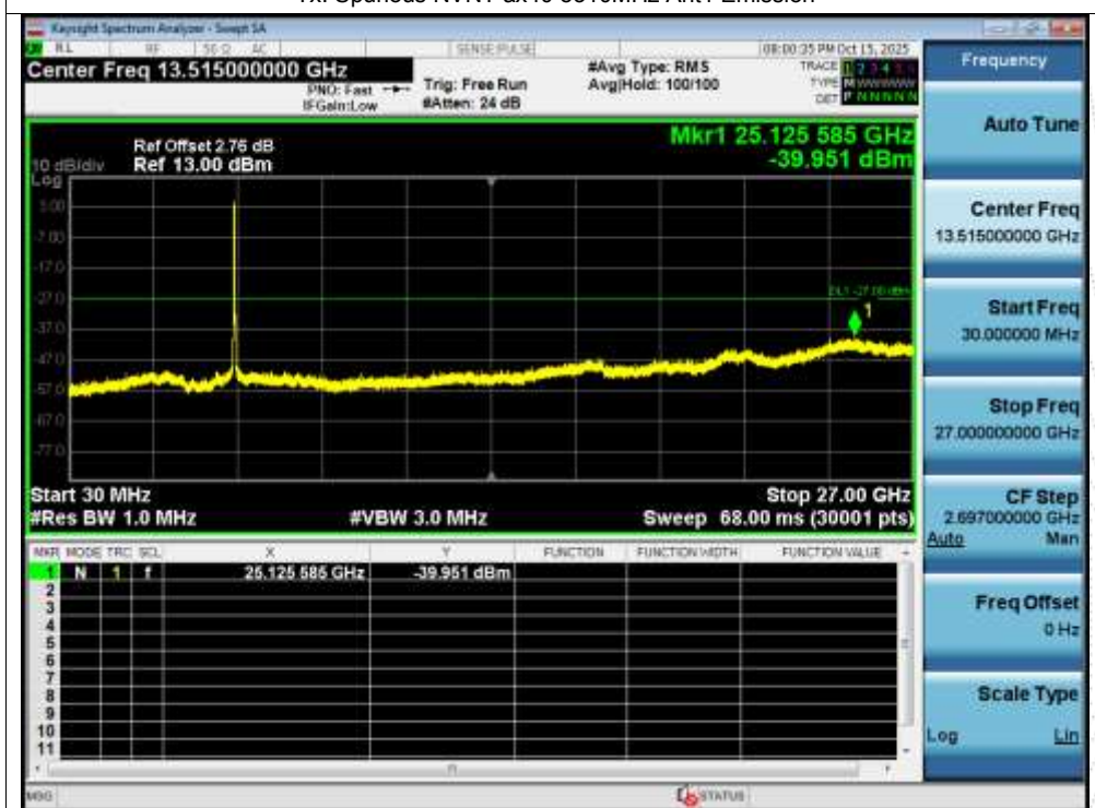
Tx. Spurious NVNT ax40 5310MHz Ant1 Emission
