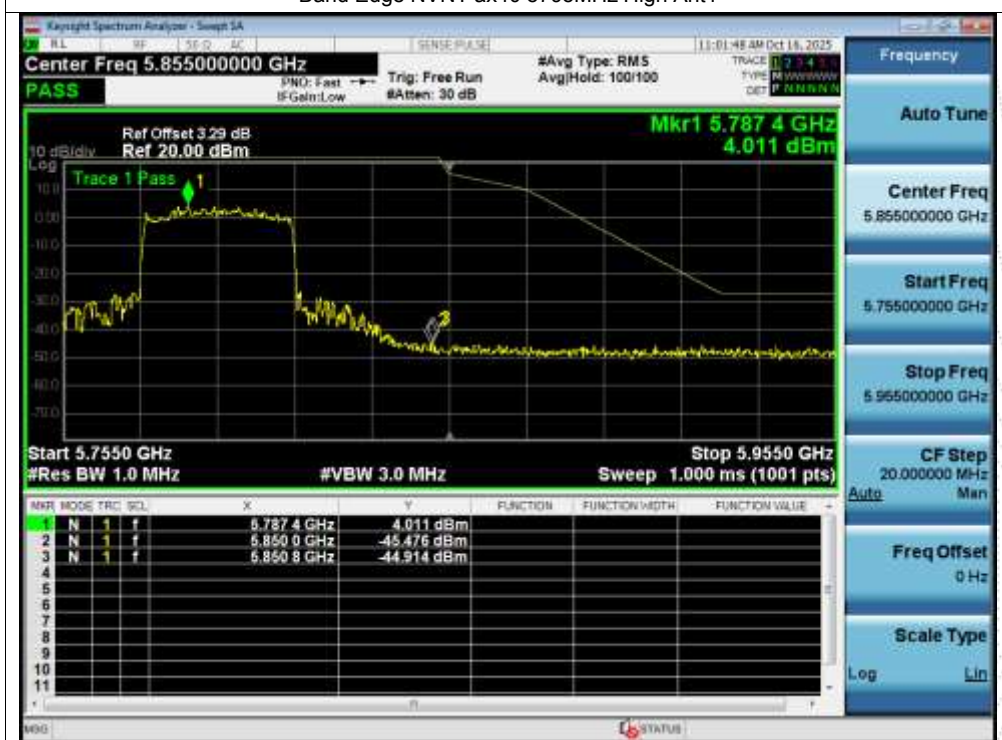
Band Edge NVNT ax40 5795MHz High Ant1
