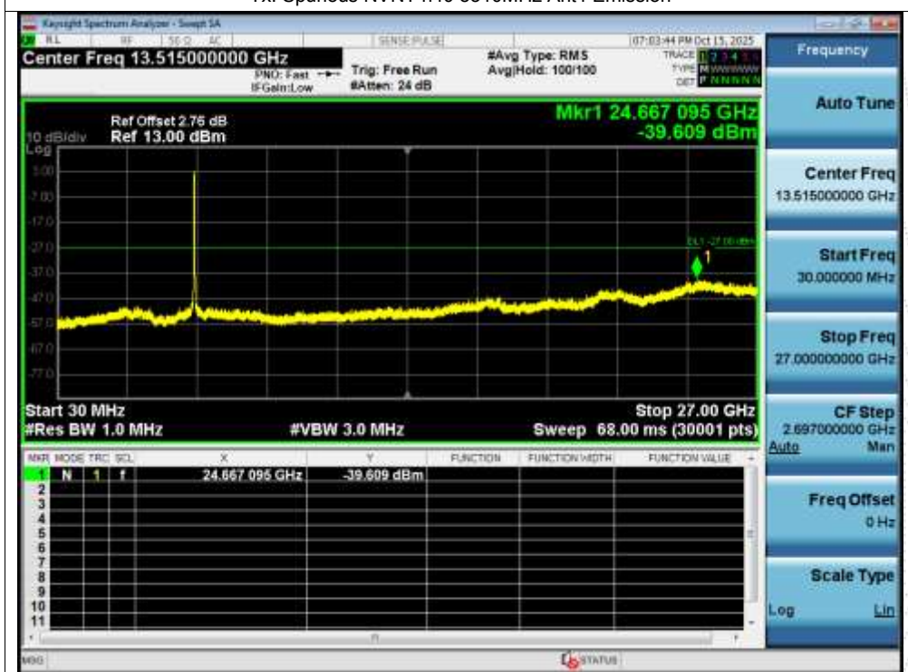
Tx. Spurious NVNT n40 5310MHz Ant1 Emission
