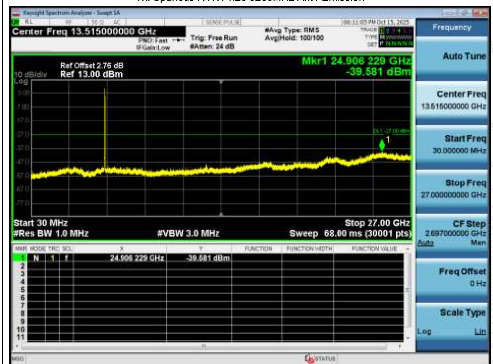
Tx. Spurious NVNT n20 5260MHz Ant1 Emission
