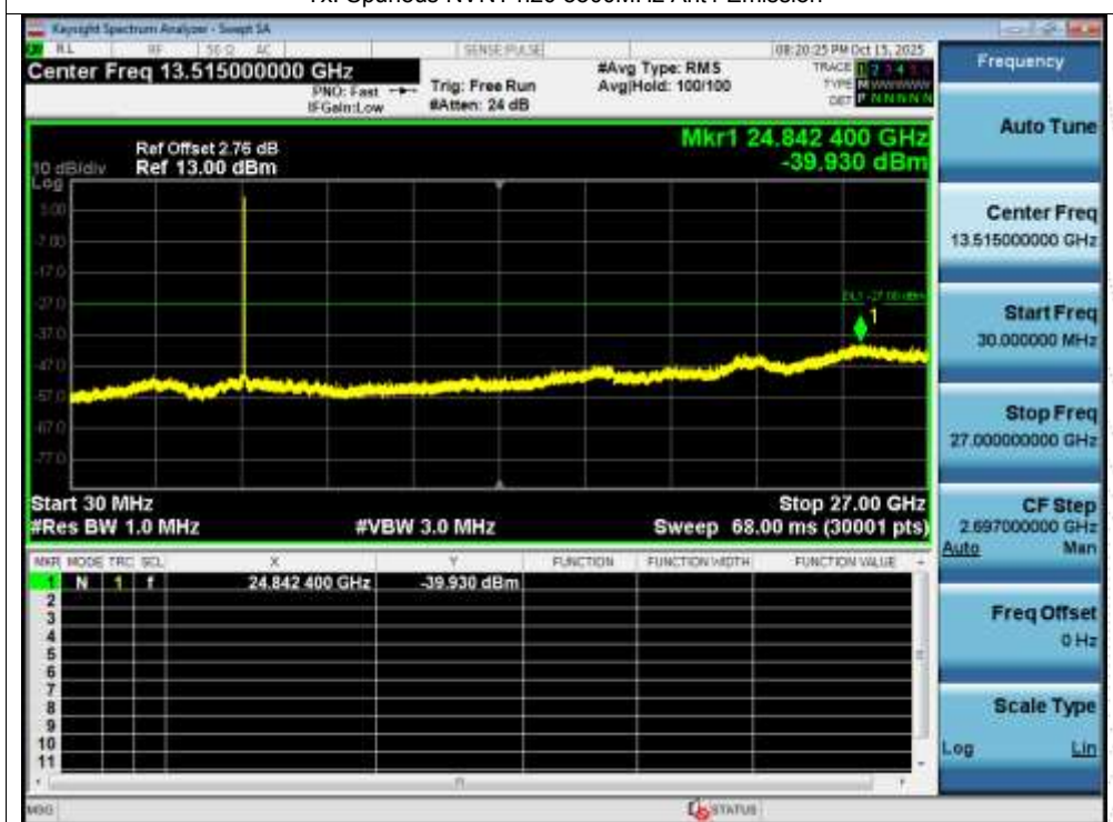
Tx. Spurious NVNT n20 5500MHz Ant1 Emission
