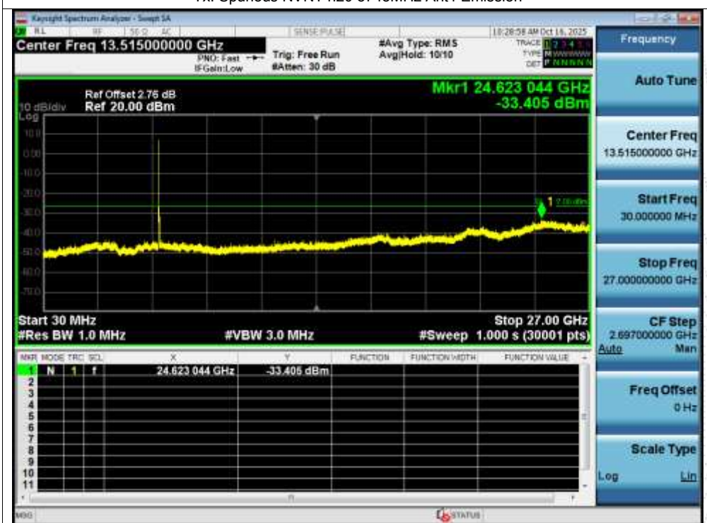
Tx. Spurious NVNT n20 5745MHz Ant1 Emission
