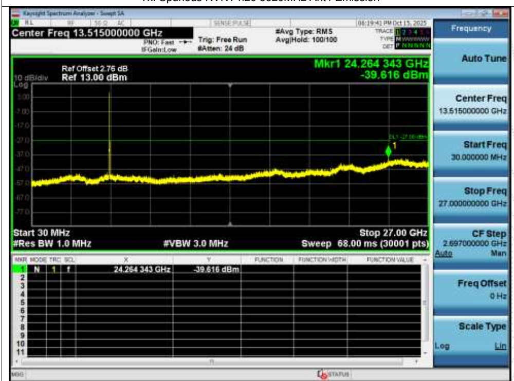
Tx. Spurious NVNT n20 5320MHz Ant1 Emission
