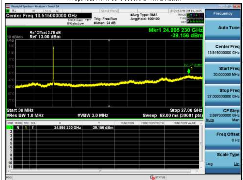
Tx. Spurious NVNT ac40 5550MHz Ant1 Emission
