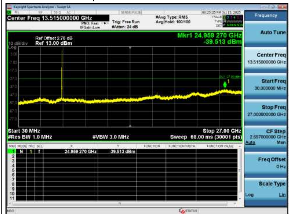
Tx. Spurious NVNT ac20 5280MHz Ant1 Emission
