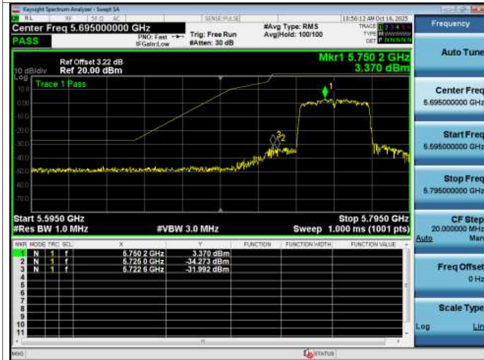
Band Edge NVNT ac40 5795MHz High Ant1
