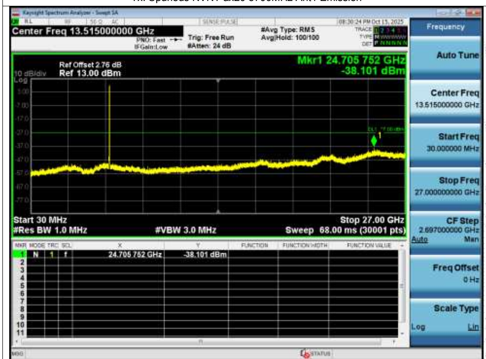
Tx. Spurious NVNT ax20 5700MHz Ant1 Emission
