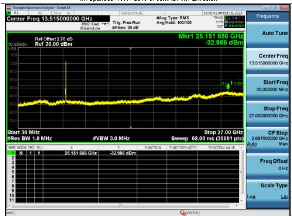
Tx. Spurious NVNT ac40 5755MHz Ant1 Emission
