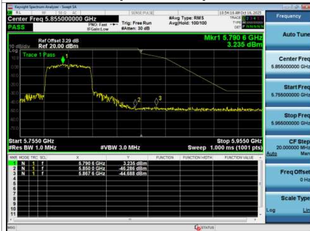
Band Edge NVNT ac40 5795MHz High Ant1
