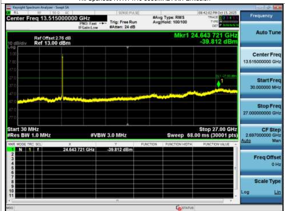
Tx. Spurious NVNT n40 5550MHz Ant1 Emission
