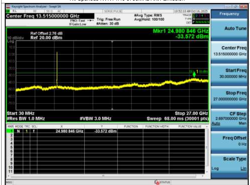
Tx. Spurious NVNT n40 5795MHz Ant1 Emission
