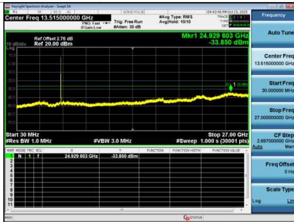
Tx. Spurious NVNT a 5200MHz Ant1 Emission
