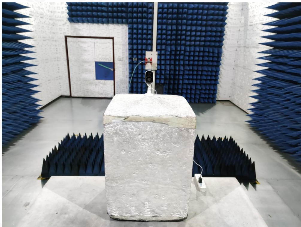
FCC RADIATED EMISSION TEST SETUP ABOVE 1GHZ
