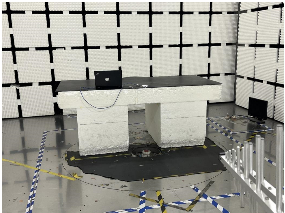
Radiation Emission Test Setup (30MHz to 1GHz)
