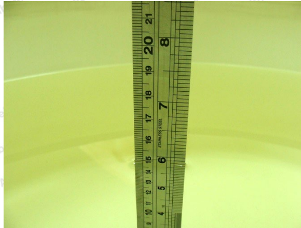
Photo of Liquid Height for Body SAR
