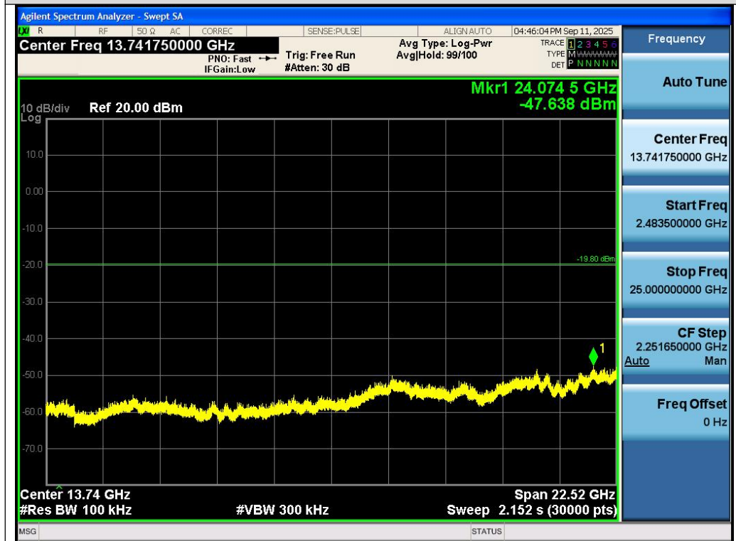
Test_Graph_802.11n20_ANT1_2412_MCS0_Higher Band Emissions
