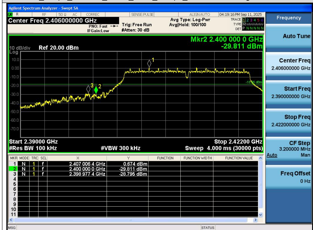
Test_Graph_802.11g_ANT1_2412_6Mbps_Lower Band Edge Emissions
