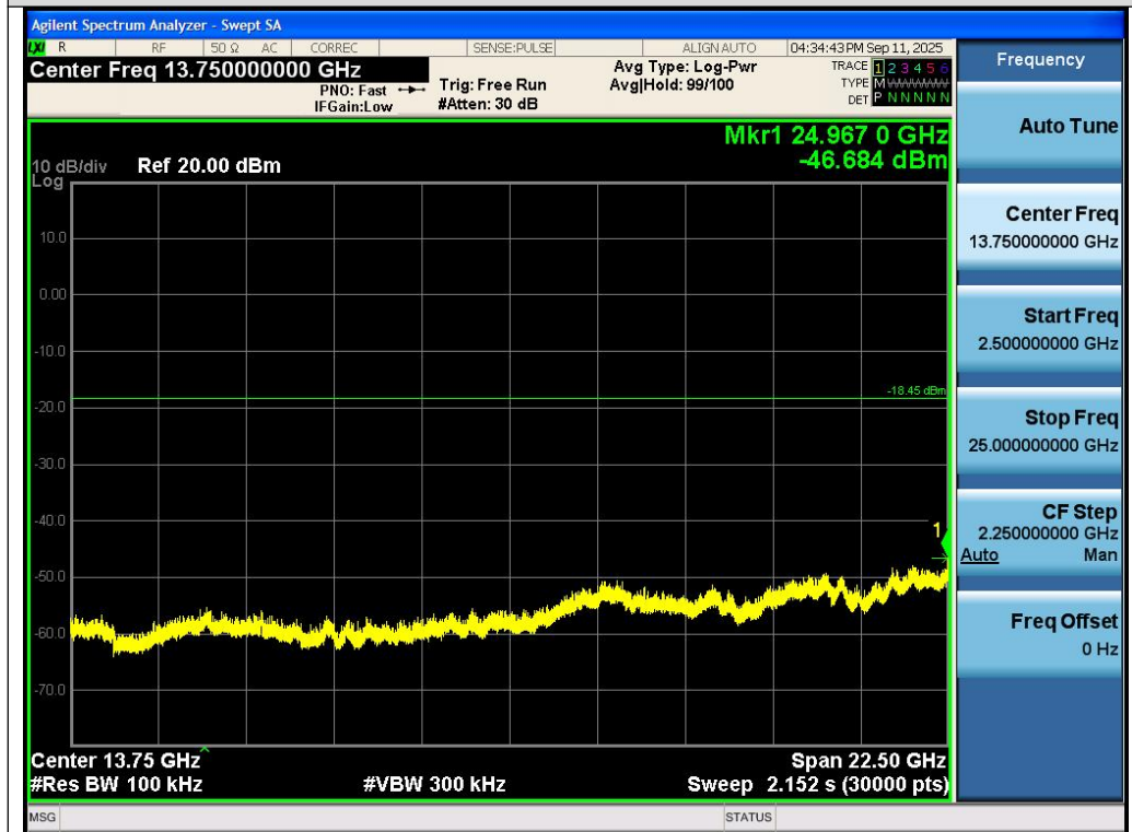
Test_Graph_802.11g_ANT1_2462_6Mbps_Higher Band Emissions
