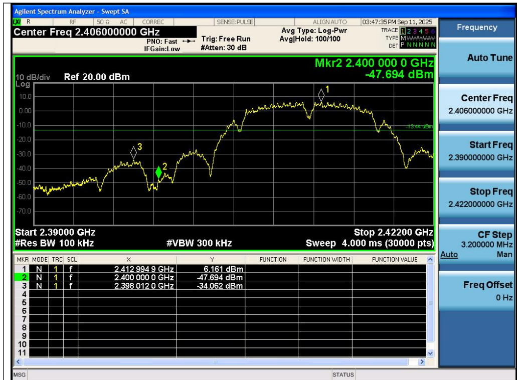
Test_Graph_802.11b_ANT1_2412_1Mbps_Lower Band Edge Emissions
