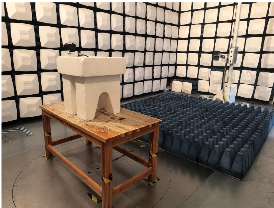
Test Setup For Radiated Emission (Above 1GHz)
