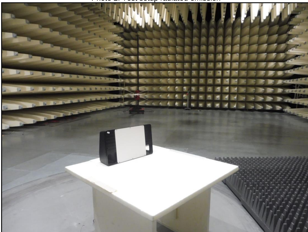
Photo 2: Test setup for radiated emission testing.
