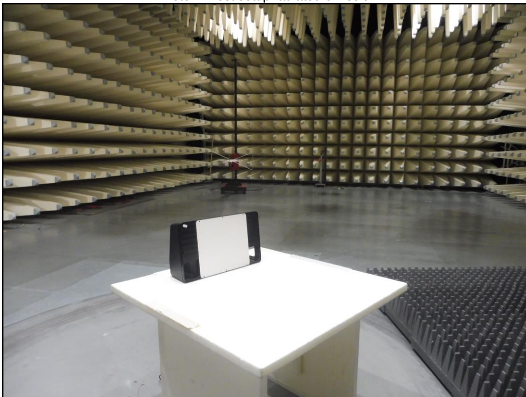
Photo 2: Test setup for radiated emission testing.
