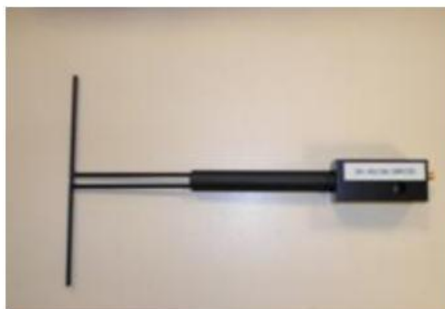
Figure 1 – Satimo COMOSAR Validation Dipole
