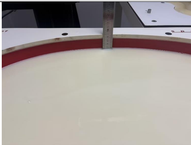
Photo 2: Tissue Simulant Liquid for Head 3000-8000
