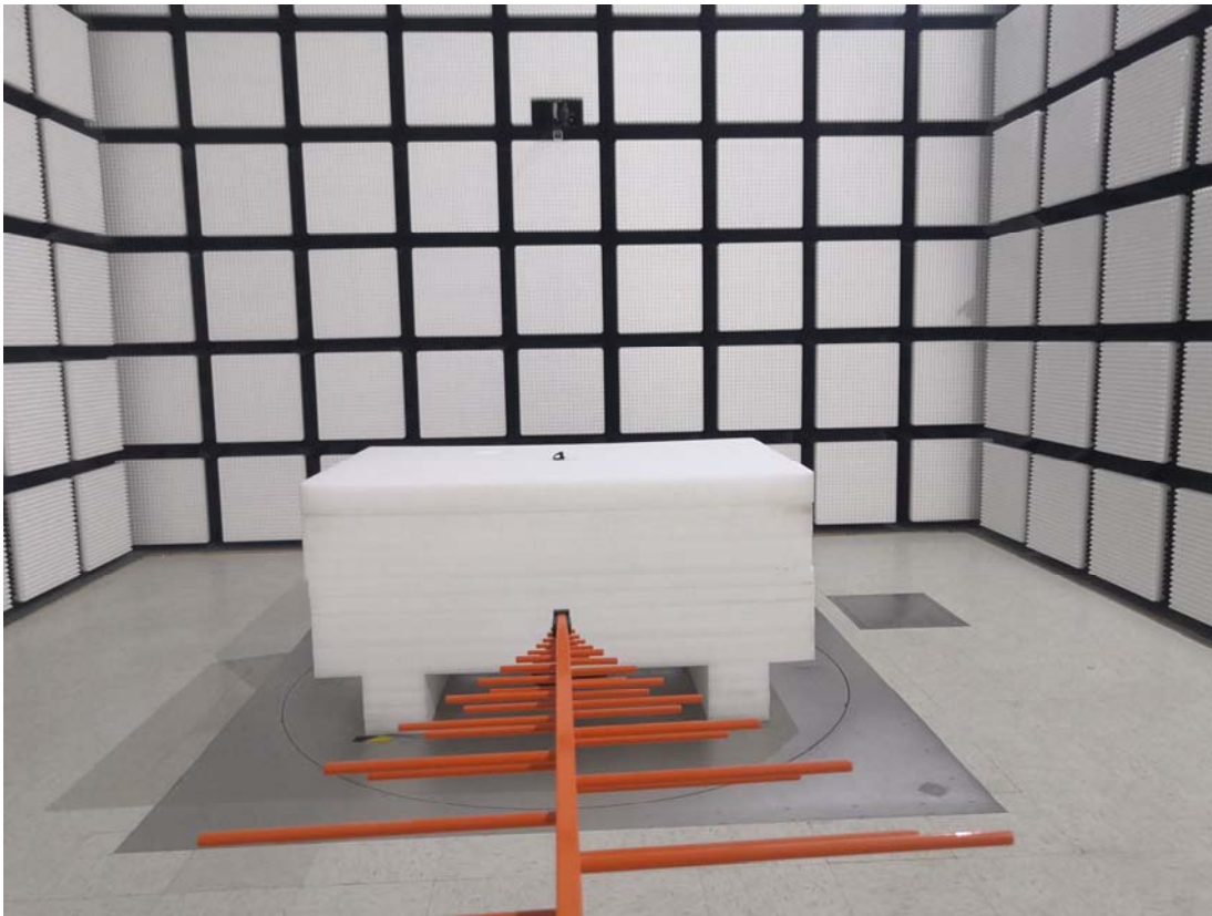
Radiated Emission Below 1GHz View
