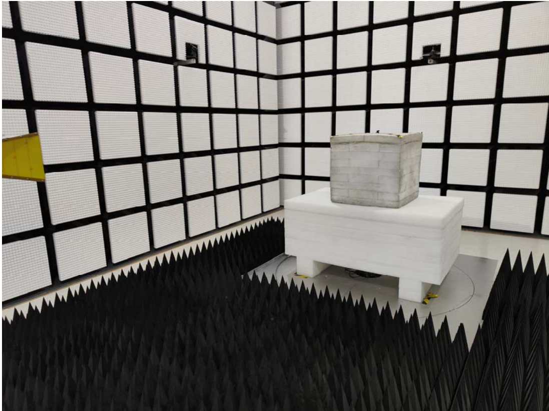
Radiated Emission Above 1GHz View
