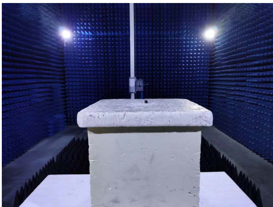
Photo of Radiated Emission Measurement Above 1GHz
