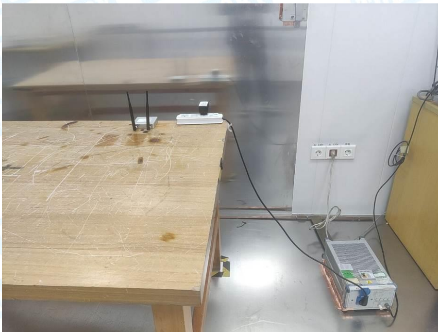
Photo of Setup for Conducted Emission
