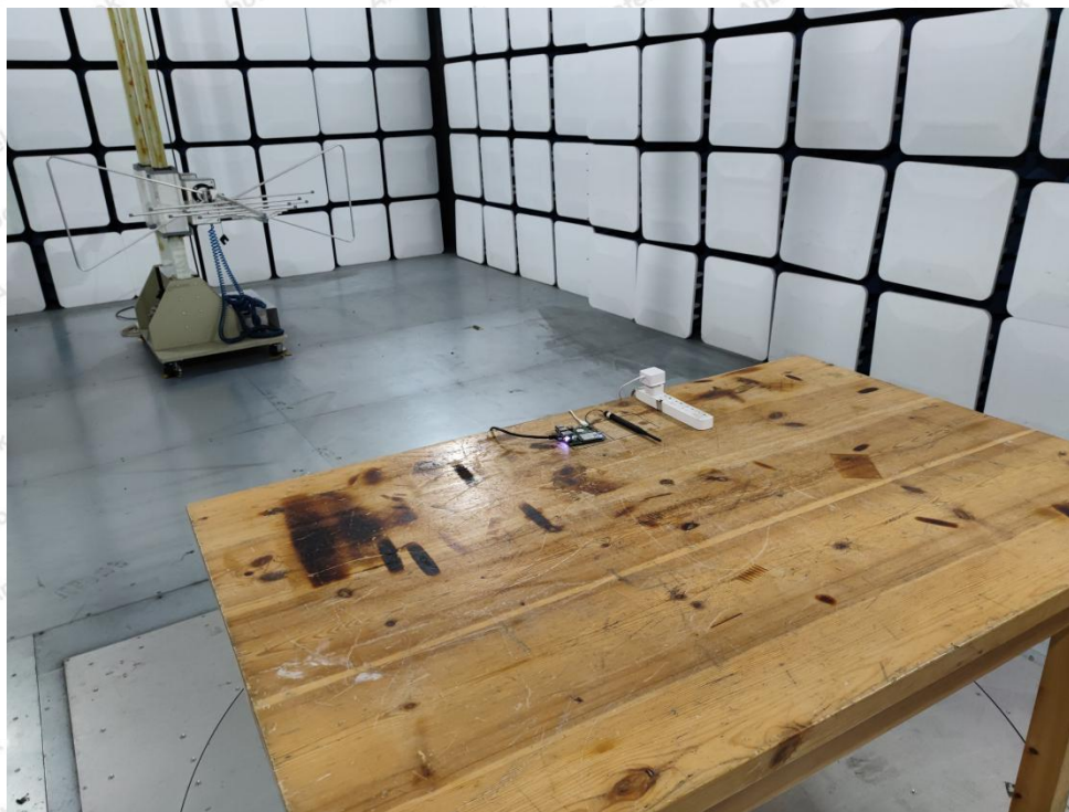
Photo of Radiation Emission Test
