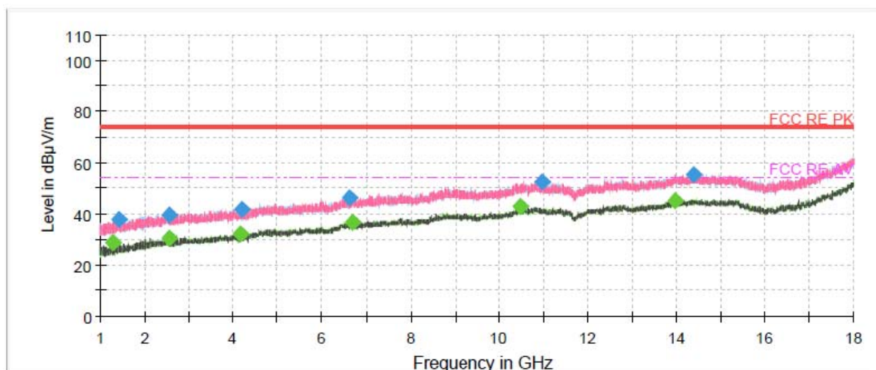
Radiated Emission from 1GHz to 18GHz
