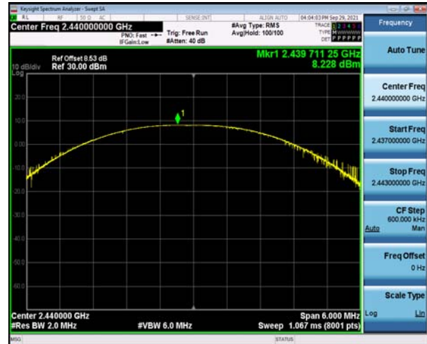
Bluetooth LE, Carrier frequency (MHz): 2440
