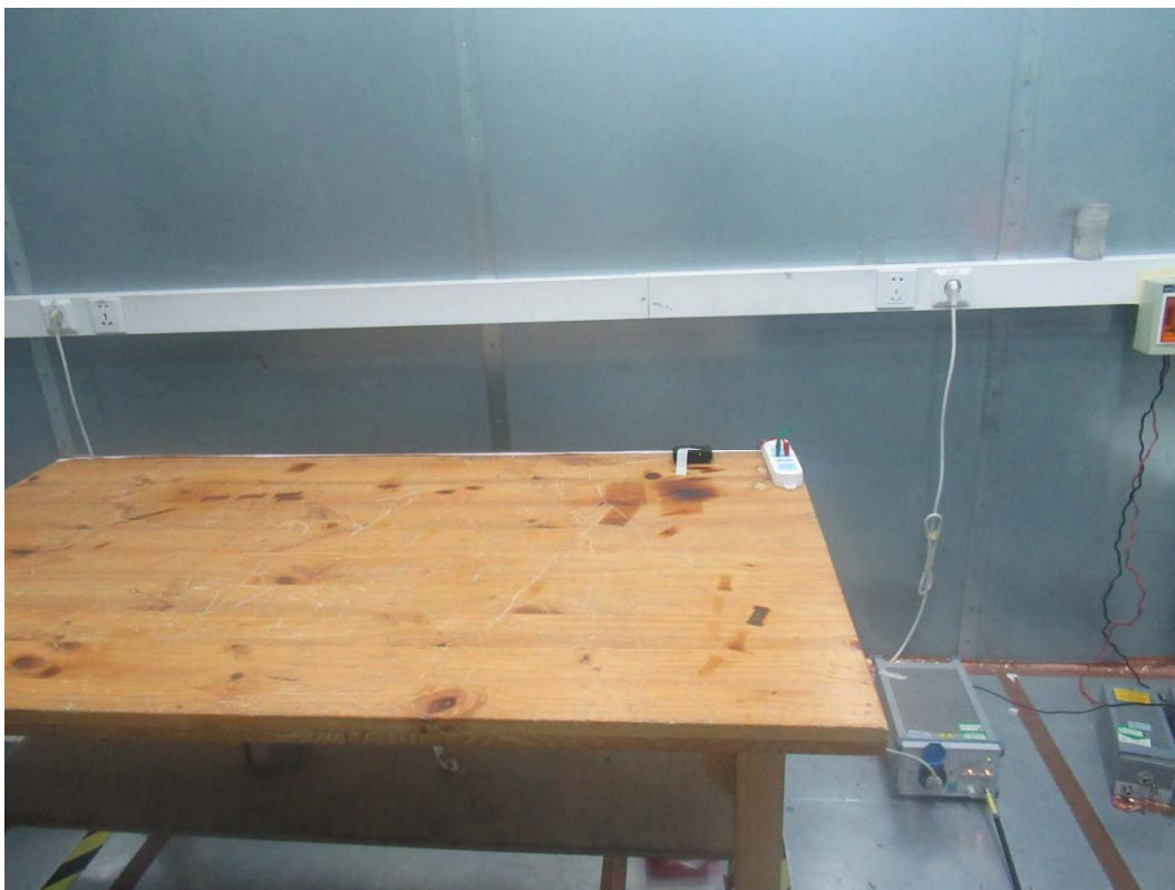
Picture 2 Conducted Emission Test Setup
