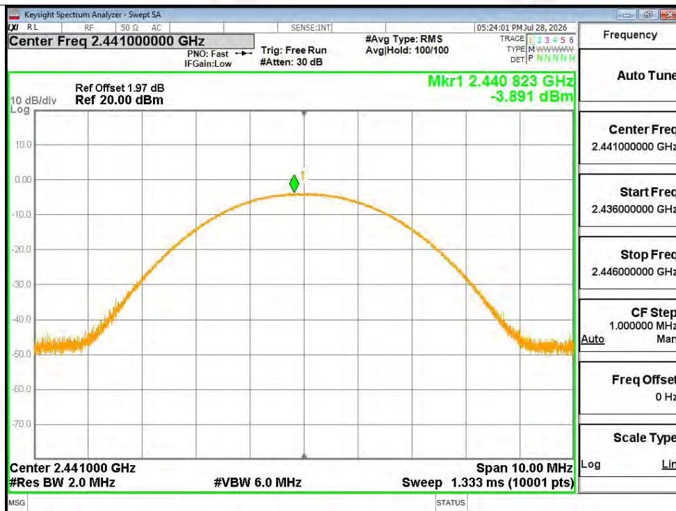
Peak Power NVNT 2-DH5 2441MHz Ant1
