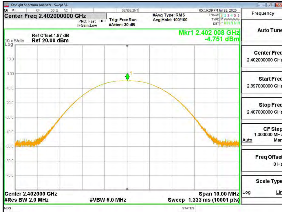
Peak Power NVNT 1-DH5 2402MHz Ant1
