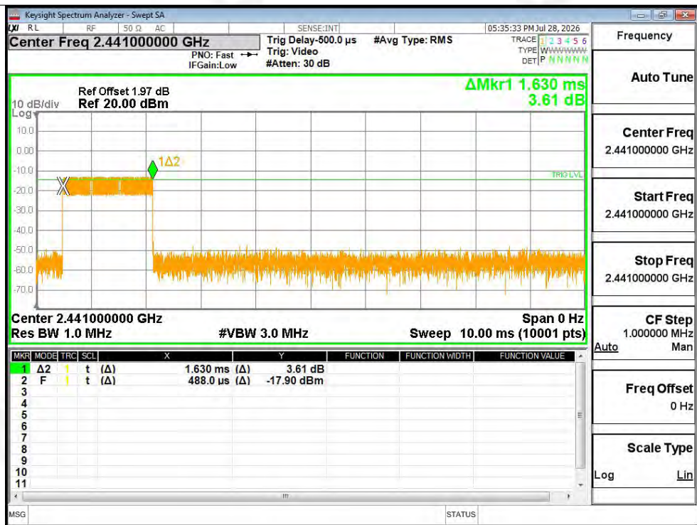
Dwell NVNT 1-DH3 2441MHz Ant1 One Burst
