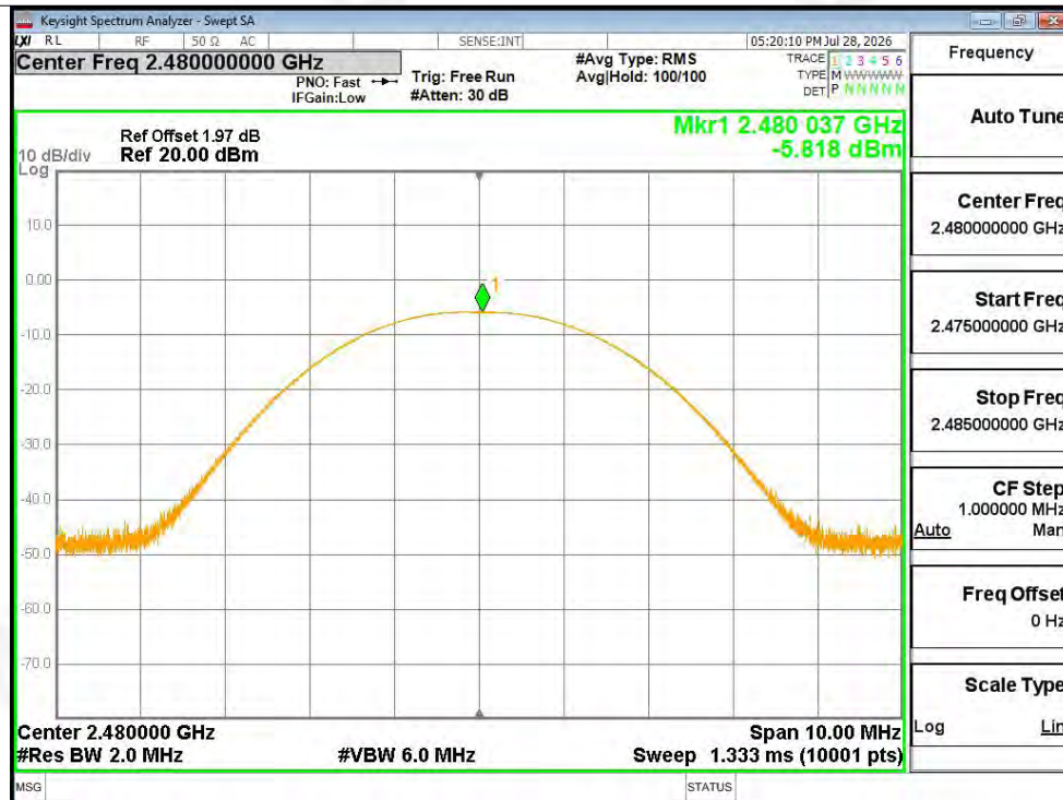
Peak Power NVNT 1-DH5 2480MHz Ant1
