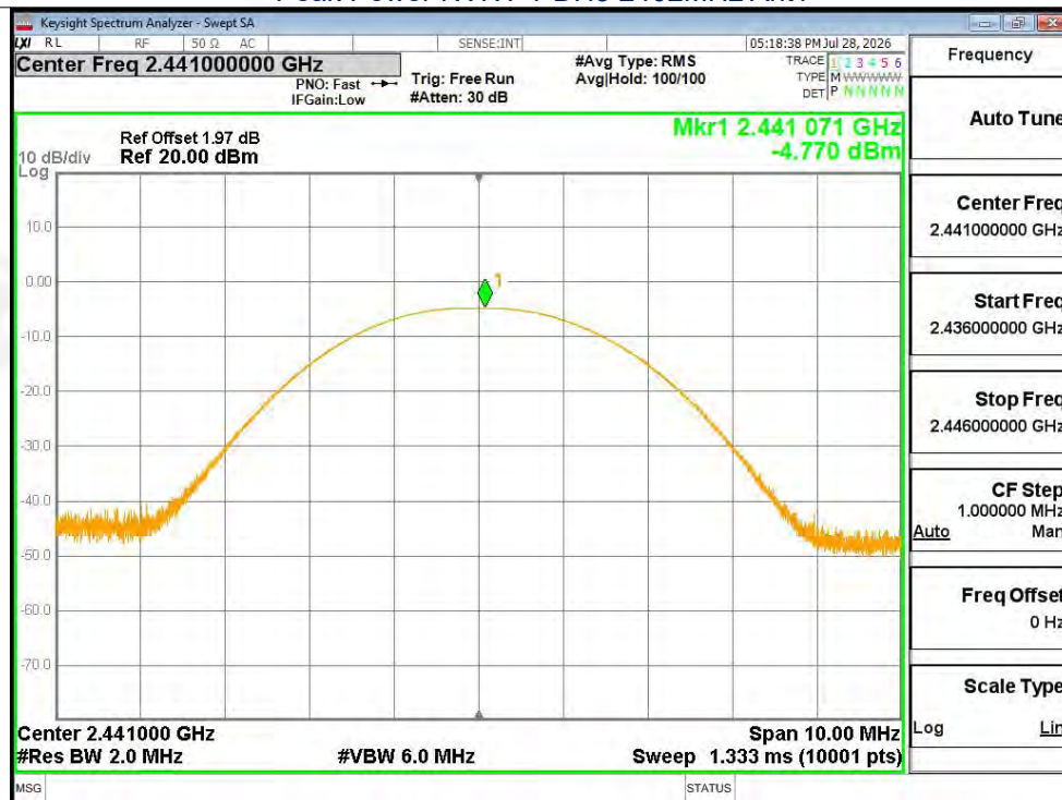
Peak Power NVNT 1-DH5 2441MHz Ant1
