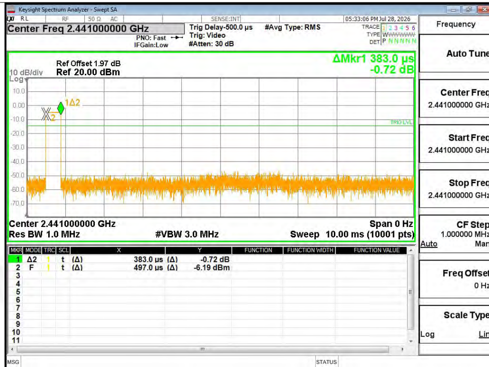
Dwell NVNT 1-DH1 2441MHz Ant1 One Burst
