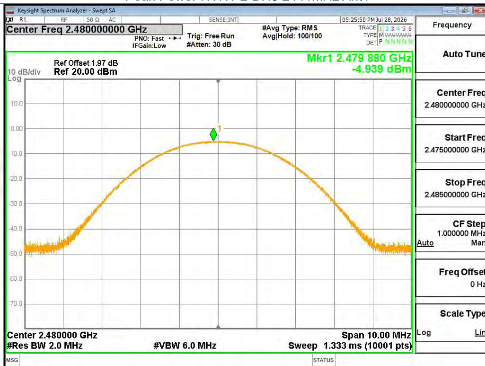
Peak Power NVNT 2-DH5 2480MHz Ant1
