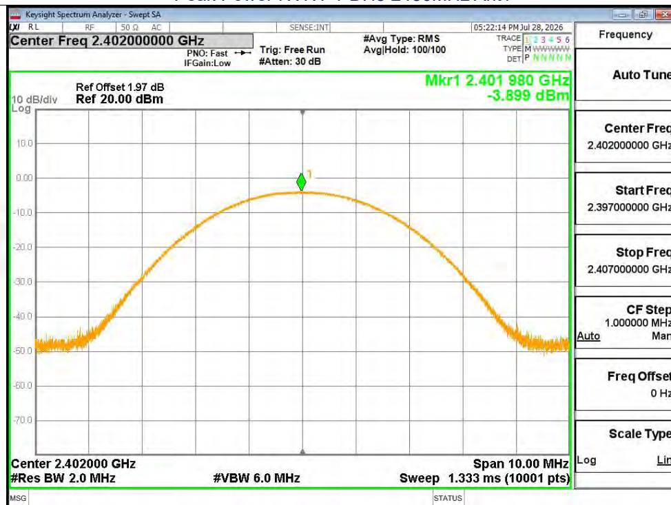
Peak Power NVNT 2-DH5 2402MHz Ant1
