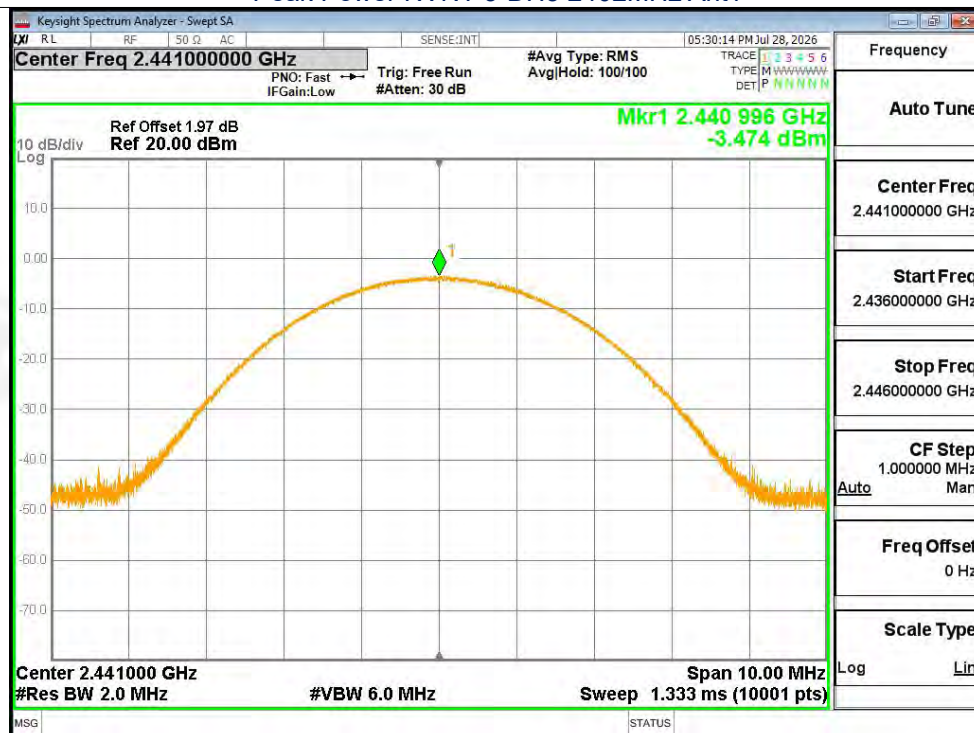
Peak Power NVNT 3-DH5 2441MHz Ant1
