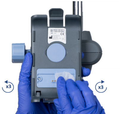
Figure 11.1. Cleaning Electric Connectors
