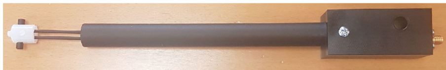
Figure 1 – MVG COMOSAR Validation Dipole
