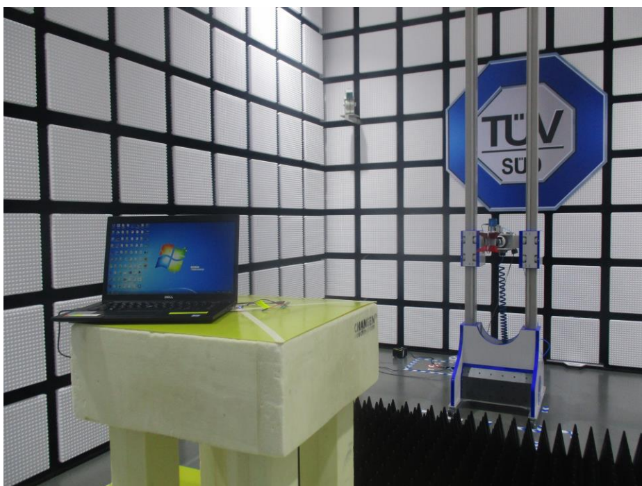
Spurious radiated emissions 1G to 18G
