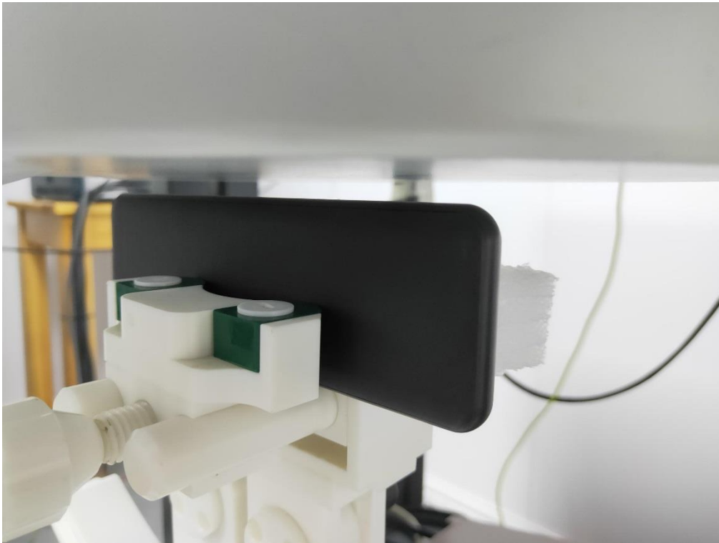
5mm body-worn Top Side Setup Photo
